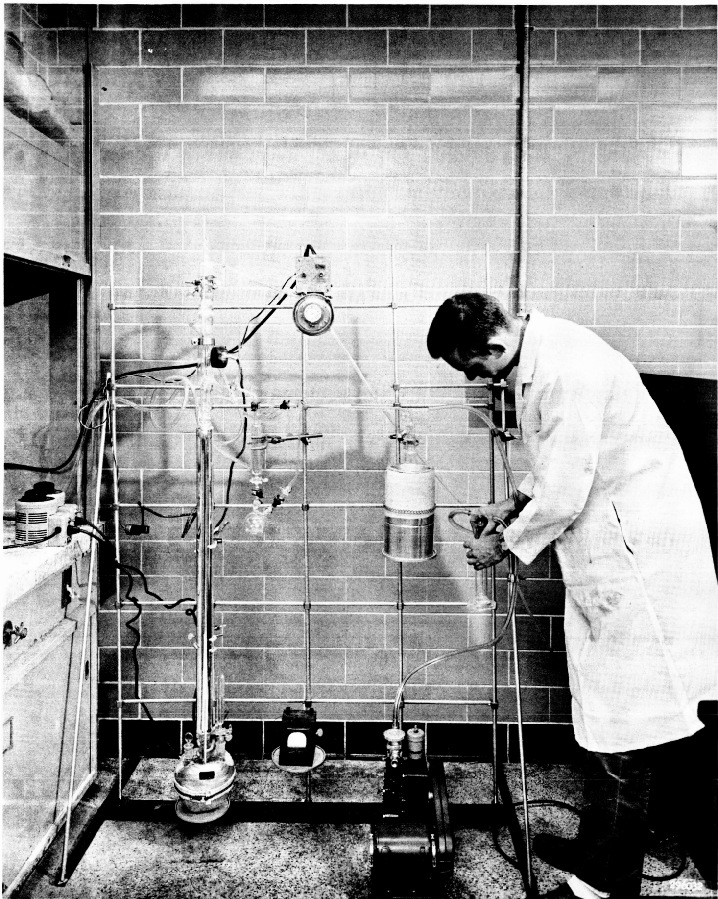
FIGURE 3. VACUUM DISTILLATION APPARATUS FOR PURIFICATION OF SOLVENTS
