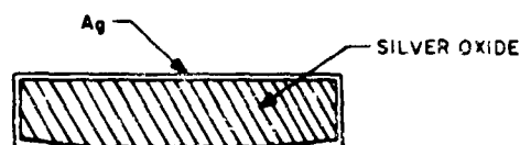
Fig. 12. Silver oxide pellet after heating at 135°C
