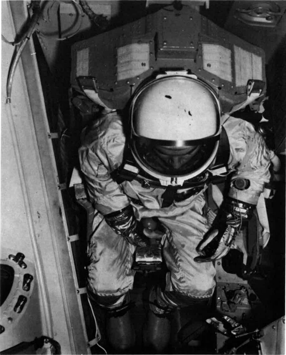
Figure 13-5.- Portable ionization chamber between legs, groin area.
