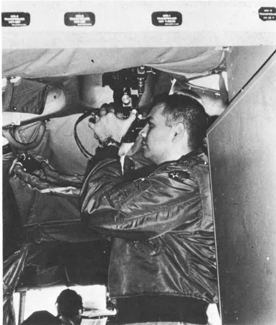
Figure 8-6.- Standard aircraft sextant to simulate orbital problem.
