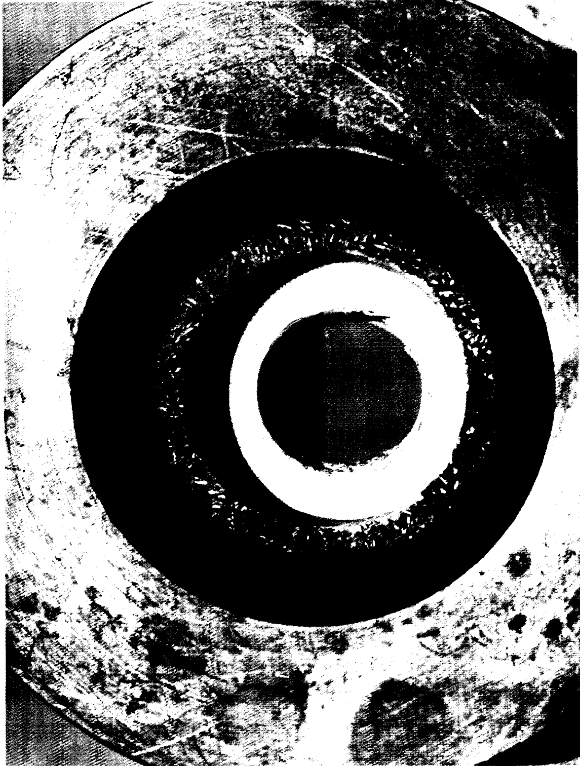
FIGURE 41. Exit End of Edge Oriented ZrC-PG Throat Insert after Run 15
