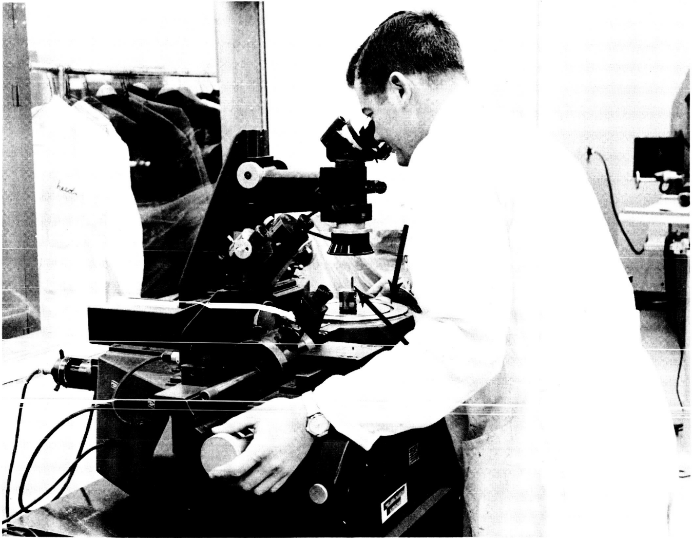
Figure 2-17 Burr point drill being inspected on Zeiss microscope with special rotary table.
