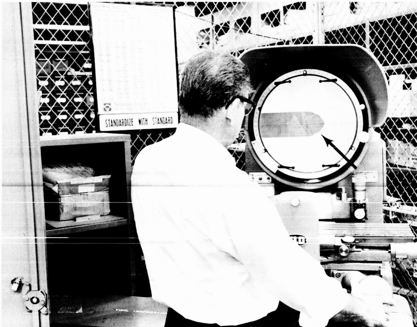
Figure 2-16 Burr point drill inspected on Excello comparator. Checking uniformity of burr gashes, depths & radius of point. (20X)
