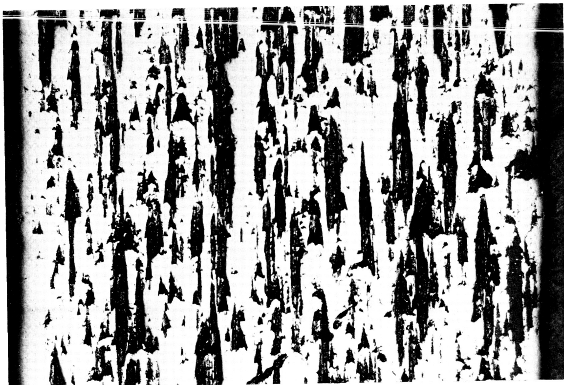
Figure 2-52 Router cut surface - lightly polished. (85X)
