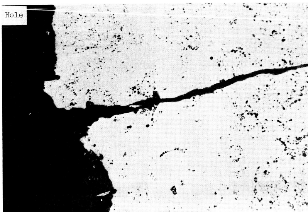
Figure 2-33 High magnification (500X) of radial crack caused by drilling hole with dull drill.(500X)
