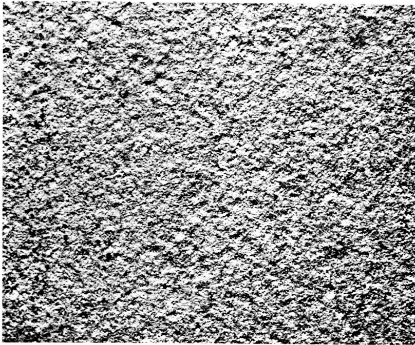
Figure 2-93 Macro photograph of Area Chemically Milled with a 45% Nitric Acid - 3% Hydrofluoric Acid Solution (Specimen #7) (18X).
