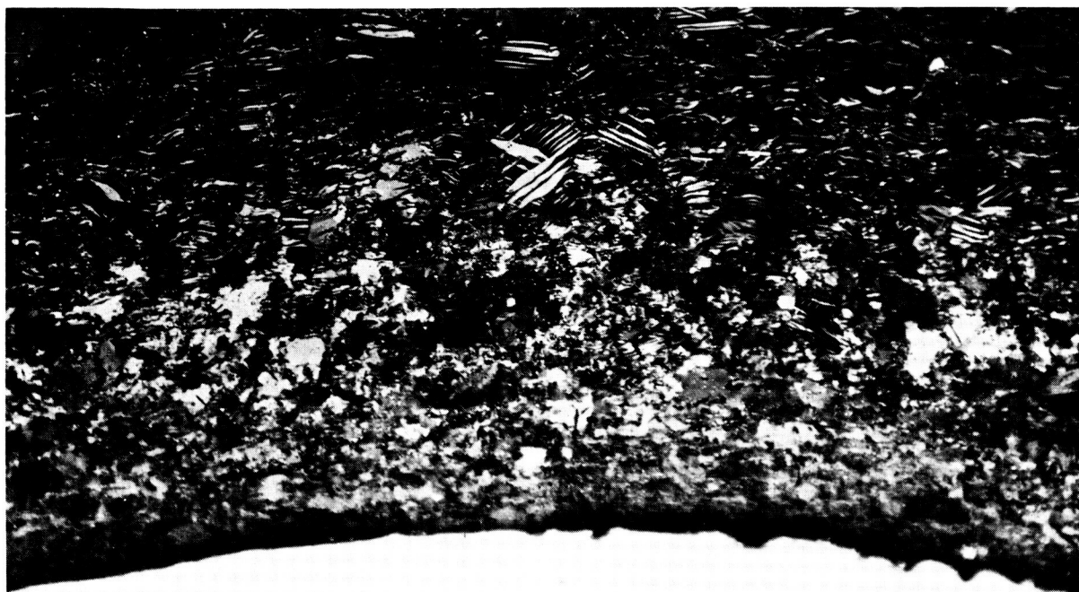
Figure 2-10 Entrance surface of punched hole showing extensive deformation twinning. (144X) Polarized Light
