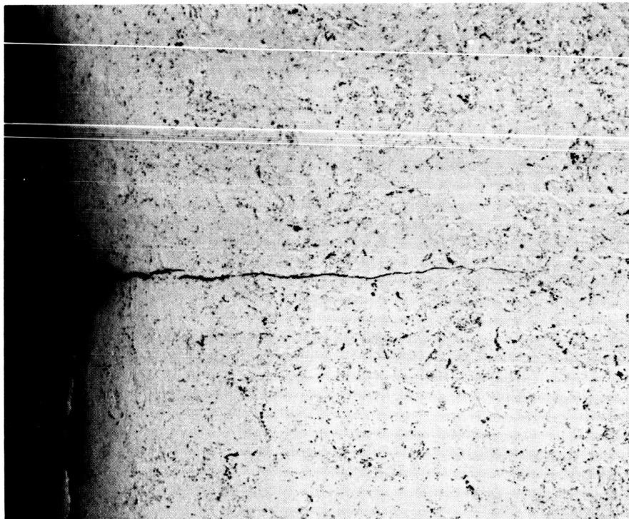
Figure 2-8 Punched & etched holes in 0.010 sheet. Photo's show extent of radial crack on entrance side & surface damage (twinning) existing even after etching. (144X)
