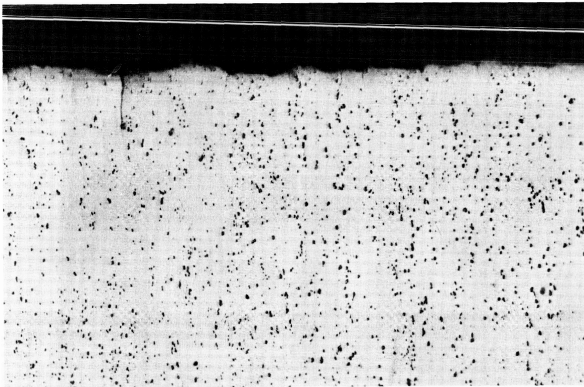
Figure 2-71 Cross-section of EDM finish cut at 32,000 CPS - metal removal rate .045 cu. in./hr. (500X)
