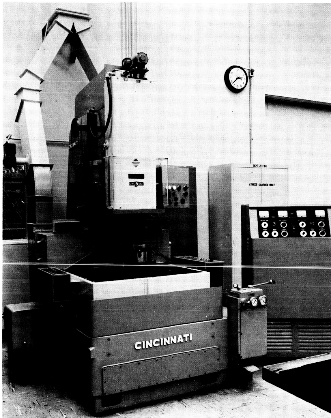
Figure 2-57 Cincinnati Model 24A31 Electrical Discharge Machine with Elox NPS D-60 power supply.
