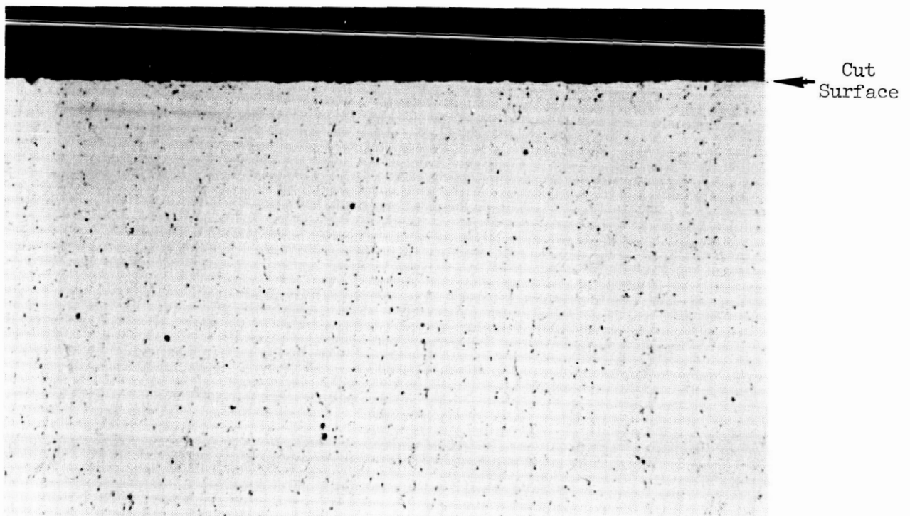
Figure 2-50 Cross-section of surface cut on abrasive wheel using coolant. Feed rate: 4.0 IPM at 8,240 SFM. (500X)
