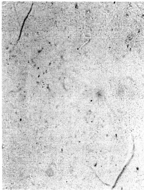
Figure IV -1. Emitter W9 after Electropolishing, 310x.
