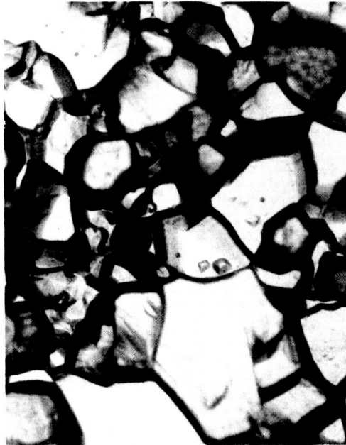
Figure IV-8. Emitter Re31 after Electroetching, 310x.
