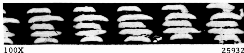
FIGURE 12. SECTIONAL VIEW OF FIVE SCREENS ELECTROFORMED ON GLASS-FILLED MANDREL IN SUPERIMPOSED POSITION
