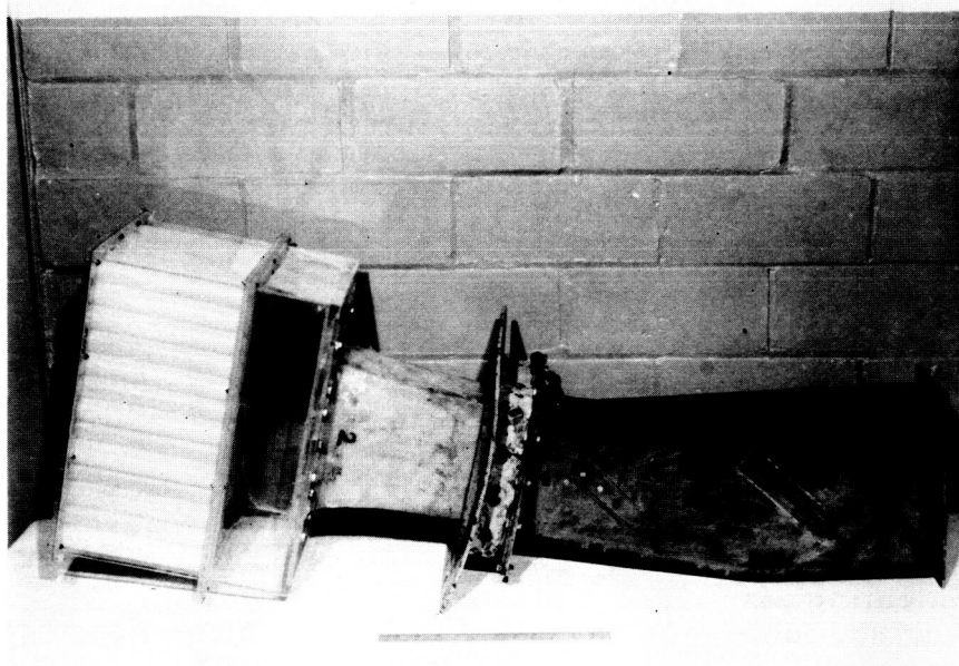
b. A test section with transition and flow straightener sections attached.
