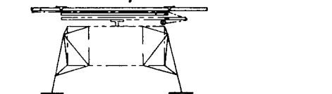
② TRACK ARMS LOWERED AND LOCKED.
