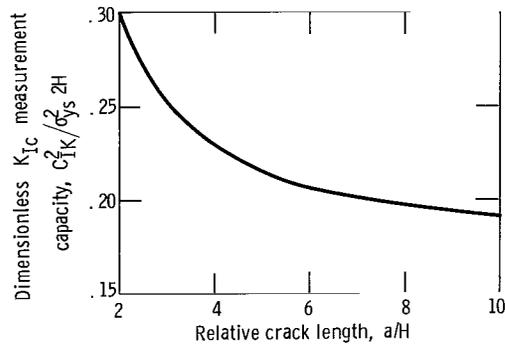
Figure 5. - Dependence of  $K_{IC}$  measurement capacity  $C_{IK}$  of single-edge-notched specimens subjected to splitting forces on relative crack length.
