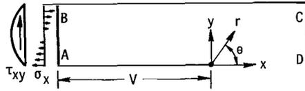
Figure 2. - Assumed equivalent distribution of boundary stresses at distance \$V\$ from end of crack.
