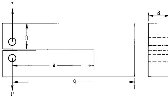
Figure 1. - Edge-cracked plate specimen subject to splitting forces.
