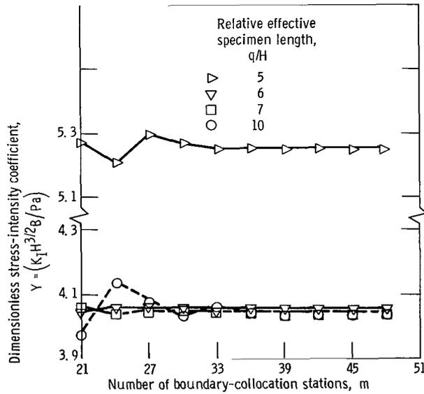
Figure 3. - Value of dimensionless stress-intensity coefficient \$Y\$ against number of boundary-collocation stations for relative crack length \$a/H = 4\$.
