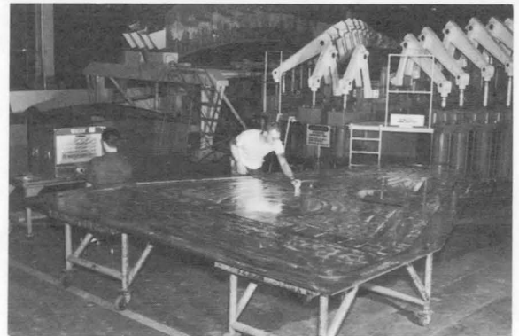
FIGURE 6.—Thickness measurements being taken on sculptured 2219 aluminum alloy gore apex prior to forming.
