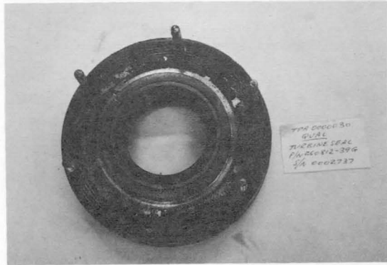
Pump Seals Life: Hot Gas Exposure - 600 Sec Propellant Exposure - 3000 Sec Typical Mode of Failure: Wear and Excessive Friction Causes Thermal Distortion
