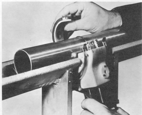
FIGURE 6.—Welding tool being clamped around tube.
