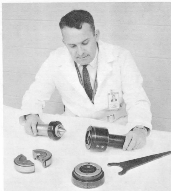
FIGURE 3.— Split die and orbital adapter. Left—Split die system; Fwd—Split-die tube clamp; Rear—Center flaring cone. Right—Orbital flaring adapter; Fwd—Iris tube chuck and spanner wrench; Rear—Orbital flaring head.
