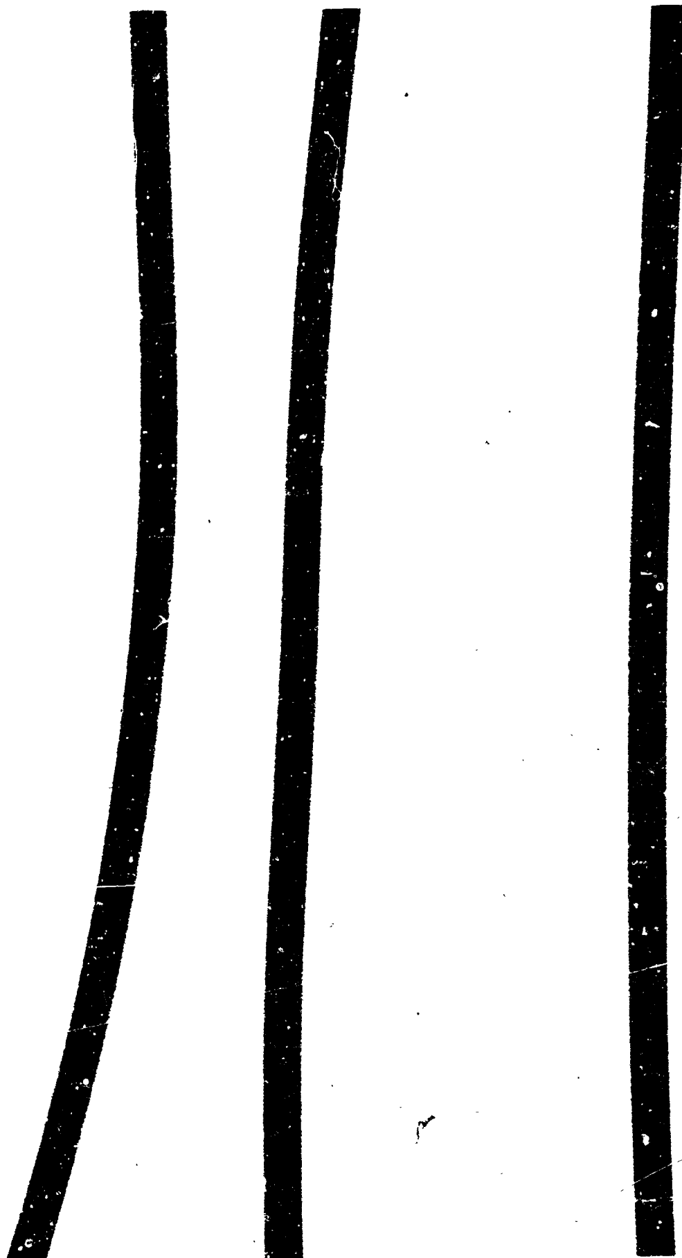
Figure 8: Typical X-ray of Wire Specimens (5X Magnification)
