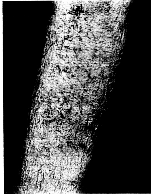
Figure A-26. Pd-25% Ag Foil Heat Treated in Air 2 Hr at 500°C. 350X
