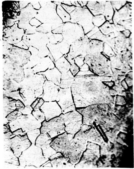
Figure A-32 Pd-25% Ag Foil Heat Treated in Air 2 Hr and in H 2 3 Hr at 600°C. 350X
