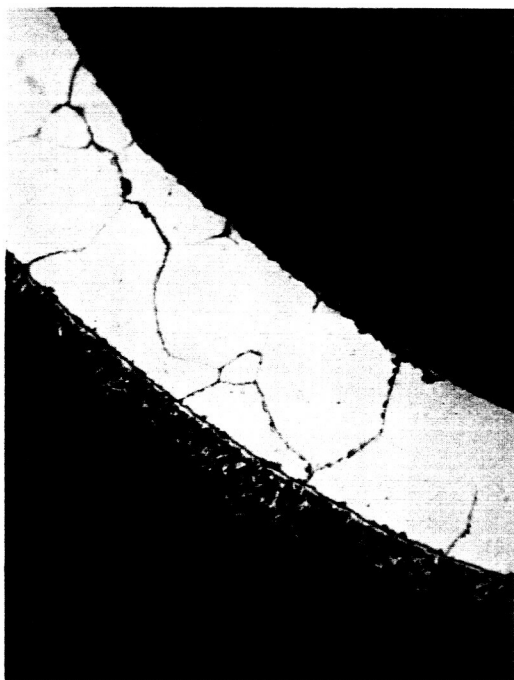
Figure A-36. Pd-25%Ag Foil Plated on Both Sides with Rh, Diffused in Argon and Oxidized in Air. After Electrochemical Tests. x500
