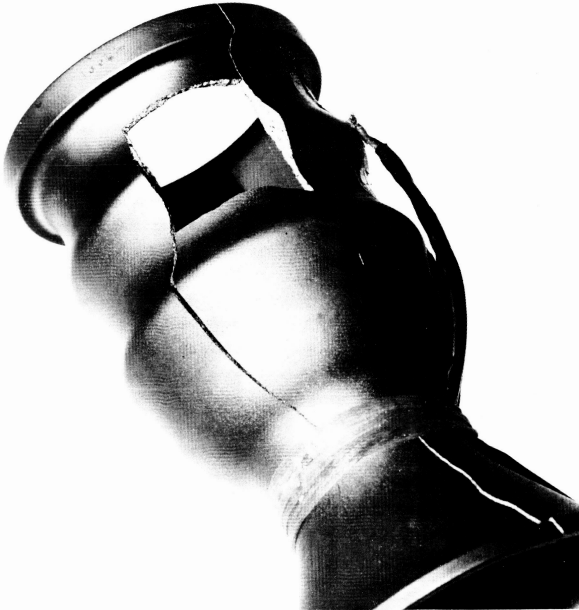
Hydrodynamically Burst Molybdenum/Durak B Chamber
