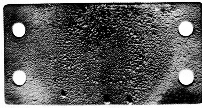
C-103/W + R508C AFTER TORCH TESTING
