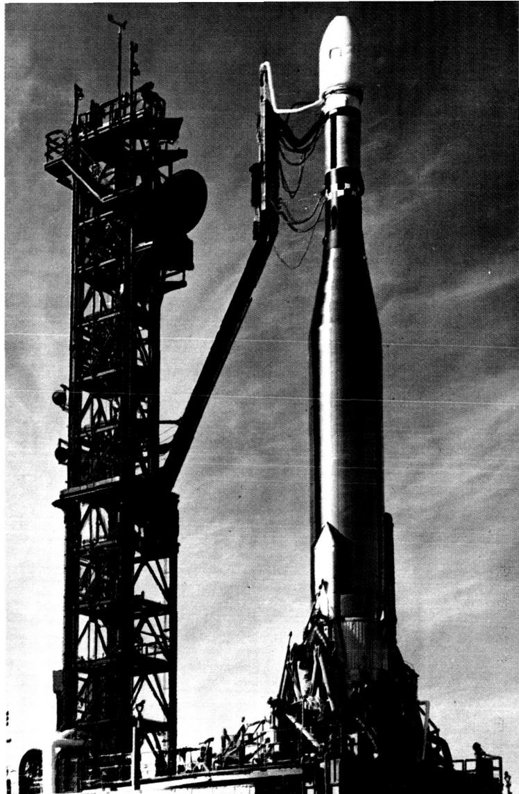
Spacecraft and launch vehicles were given separate system tests, assuring that each would function in every phase of its role in the mission. The mechanical, electrical, and radio compatibility of spacecraft, vehicle, ground equipment, and tracking system were tested. Finally, at the beginning of November, the Mariner III spacecraft and launch vehicle stood on the pad, going through a dress rehearsal. The actual Mars launch period opened on November 4 and lasted for only about a month.
