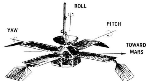
There are Sun sensors on Mariner's upper and lower decks; their output signals drive control-amplifier chains, which use puffs of nitrogen gas from paired jets on the tips of the solar panels to turn the spacecraft until the panels face the Sun, and to stop it in that position. This process took 12 minutes.
