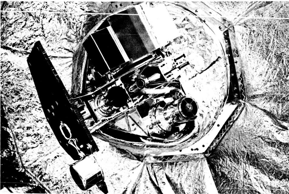
*For the first 2½ months of flight, TV optics (lower center, pointing right) and planet sensors were protected by a metal cover (shown hinged to left and down); on February 11, the cover was unlocked and pivoted open by command from Earth.*
