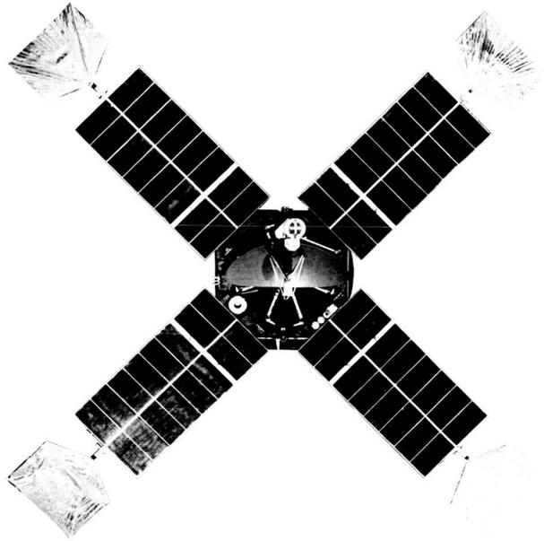
flight test; they were designed to balance the spacecraft against the endless pressure of sunlight, saving attitude-control-jet gas and permitting a longer stable flight.
