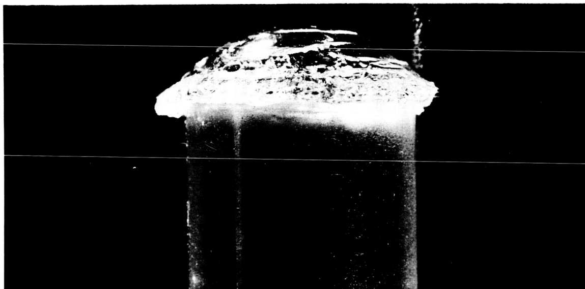
FIG. 3. GLASS ROD ABLATED IN AN ARC-JET FACILITY.
