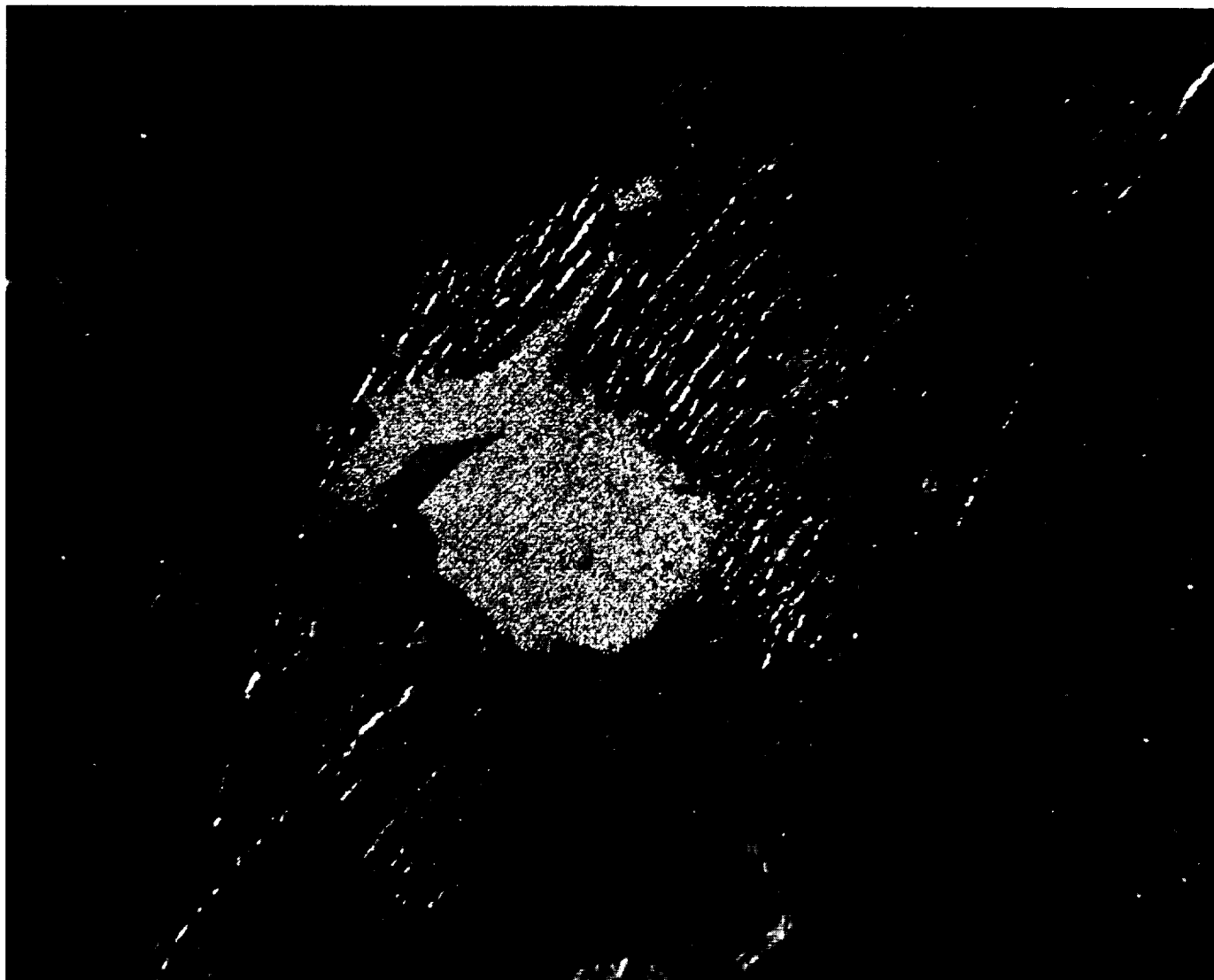
Fig. 3. Faulty area of cobalt-plated Mylar belt (85 times actual size)
