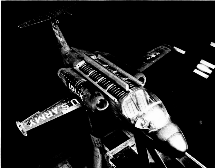
Figure 3.- The LTV XC-142 model mounted in the Ames 40- by 80-Foot Wind Tunnel (model wind-tunnel geometry in table I).
