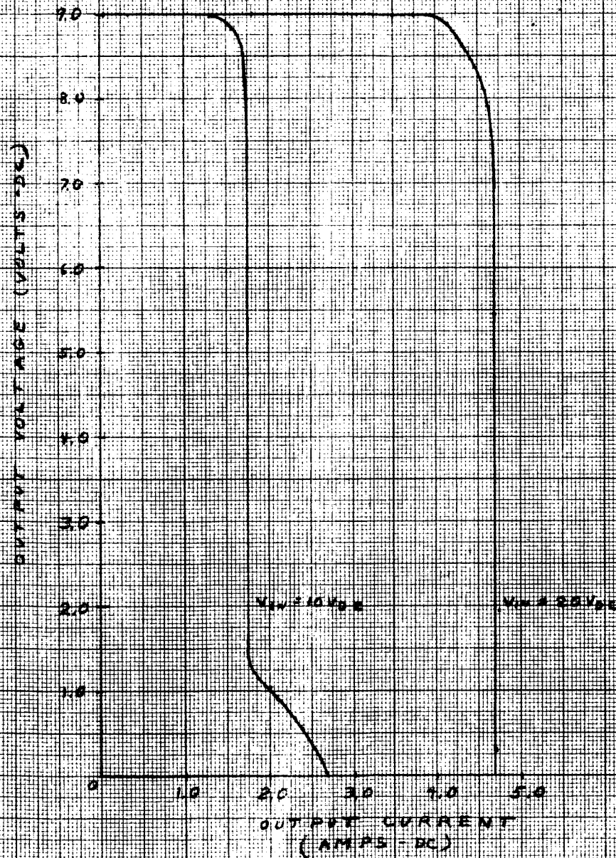
FIGURE I - 9 OVERLOAD AND SHORT CIRCUIT CHARACTERISTIC 10 WATT CHOPPER
