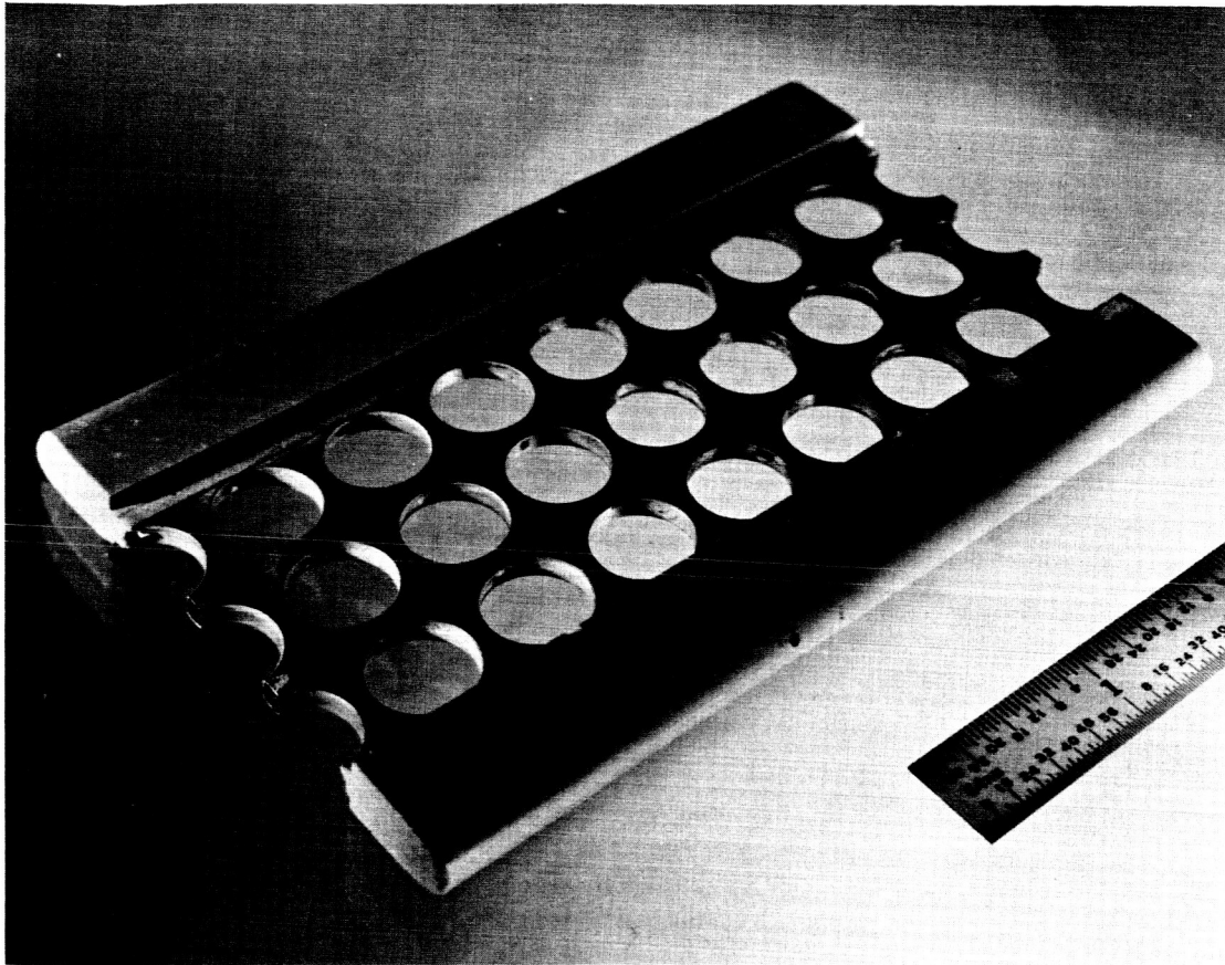
FIG. 9-16 NICKEL HOLLOW CORE BUCKLING SPECIMEN READY FOR TEST
