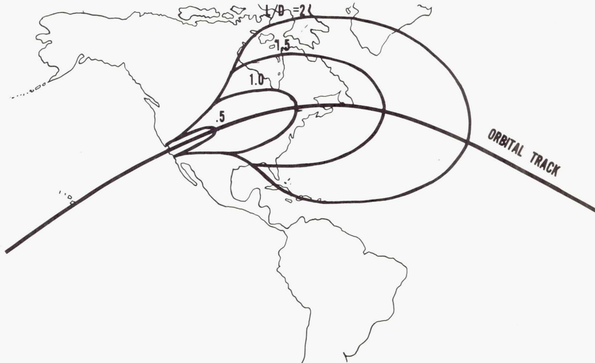
FIGURE 3.—Range capability in relation to hypersonic lift-drag ratio.
