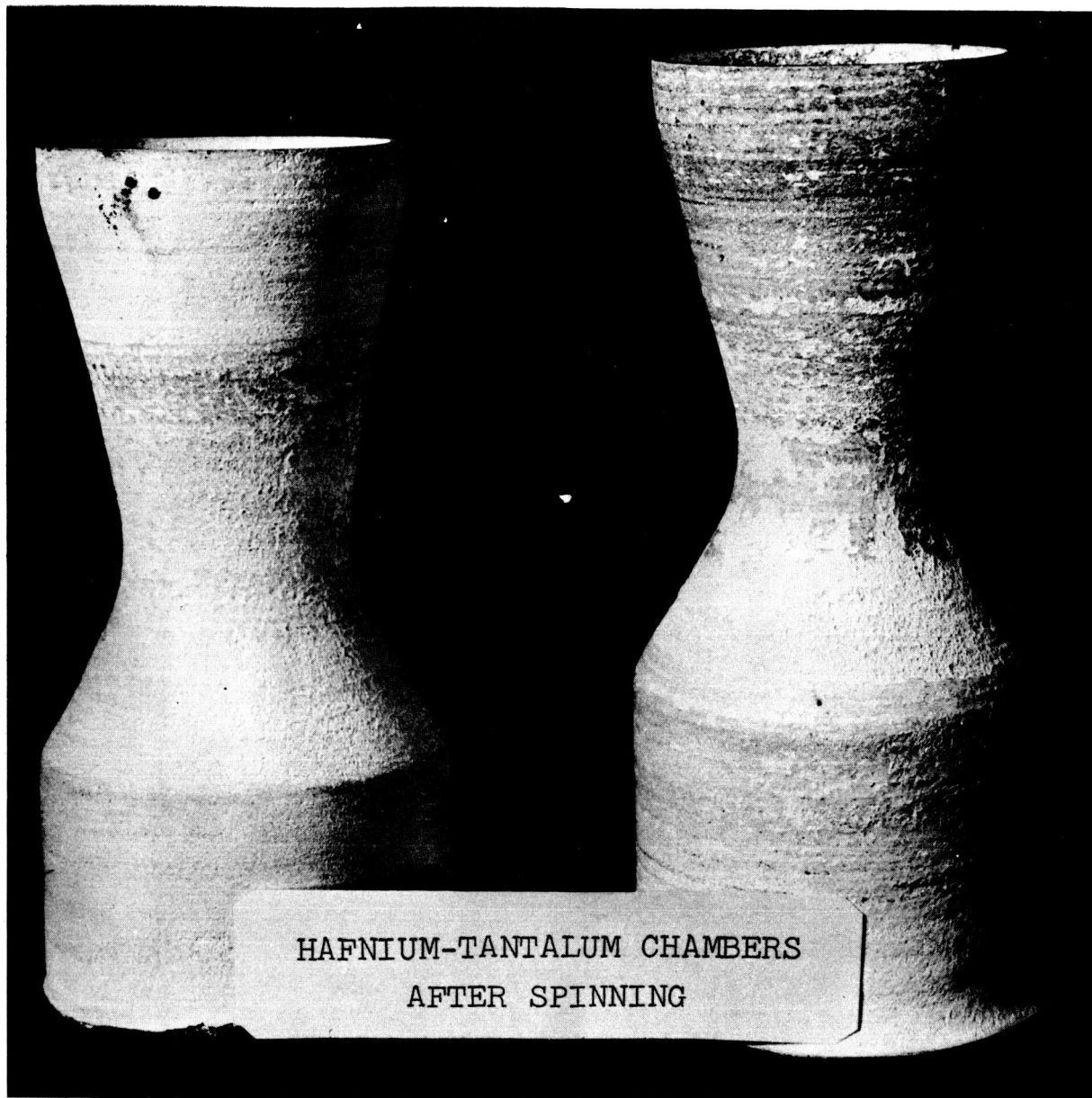
Figure V-148. Hafnium - Tantalum Chambers After Spinning
