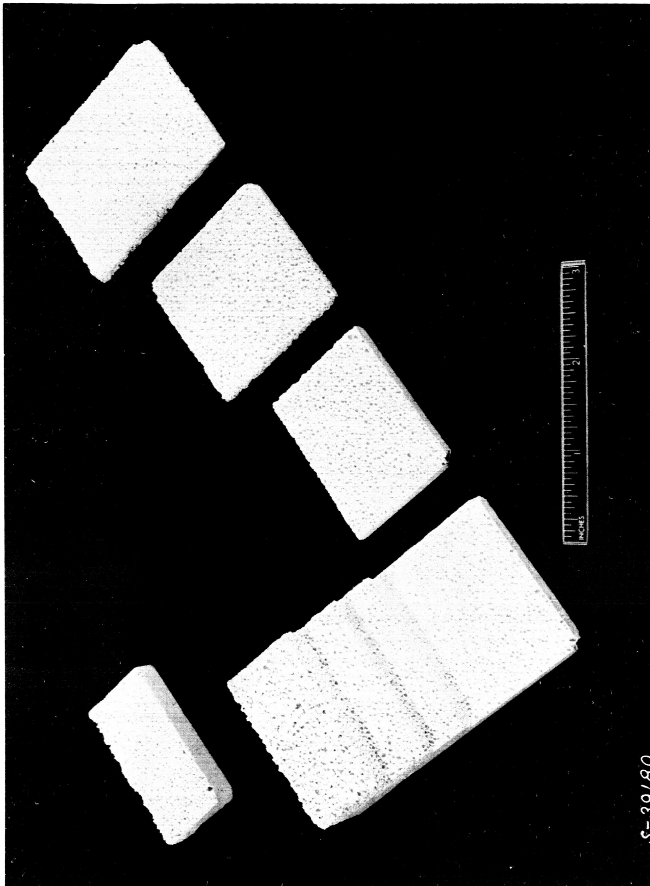
Figure 2. Foam Ceramic Body Showing Internal Structure
