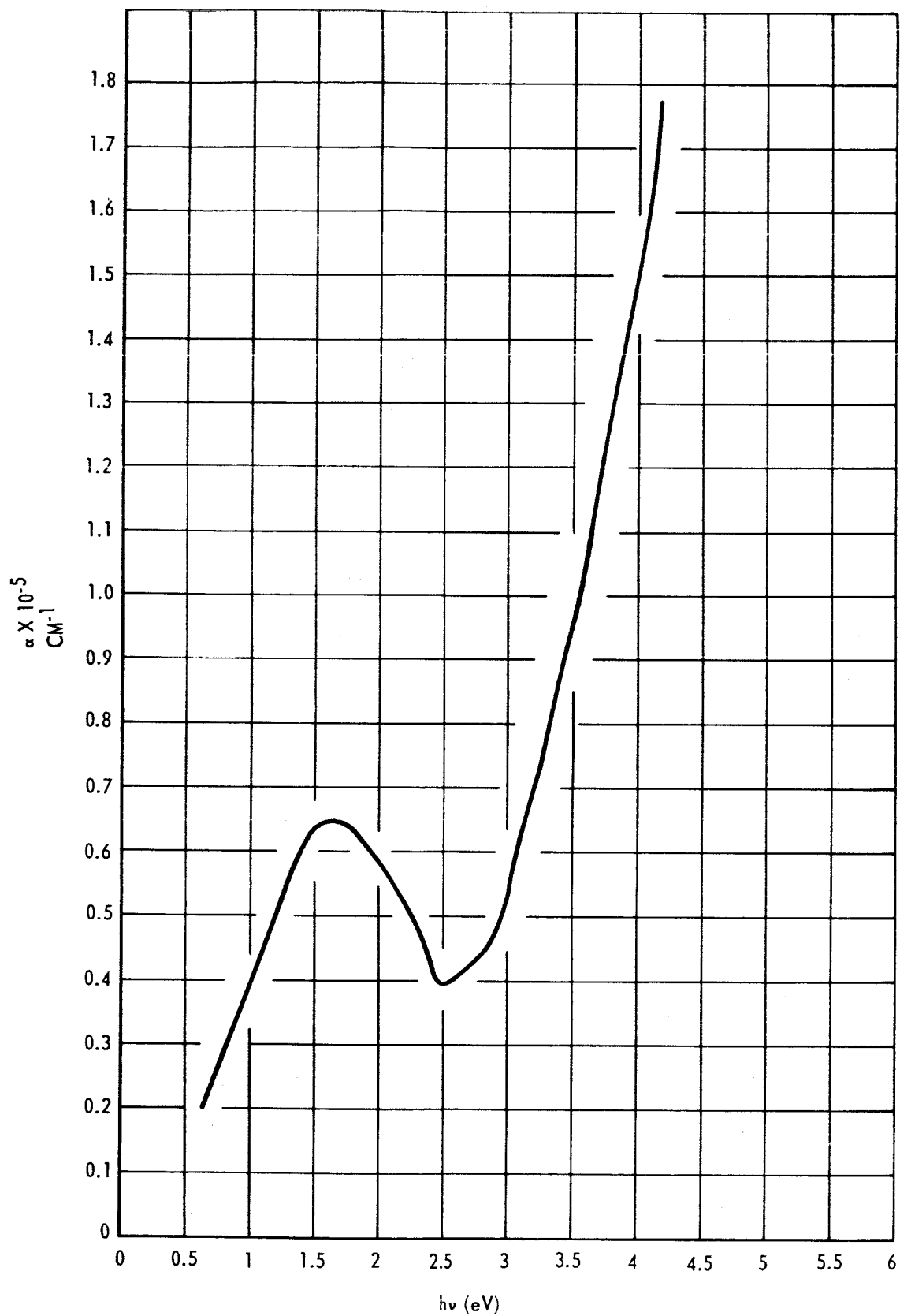
Figure 4. Absorption Coefficient \alpha of a Thin Boron Film as a Function of Energy
