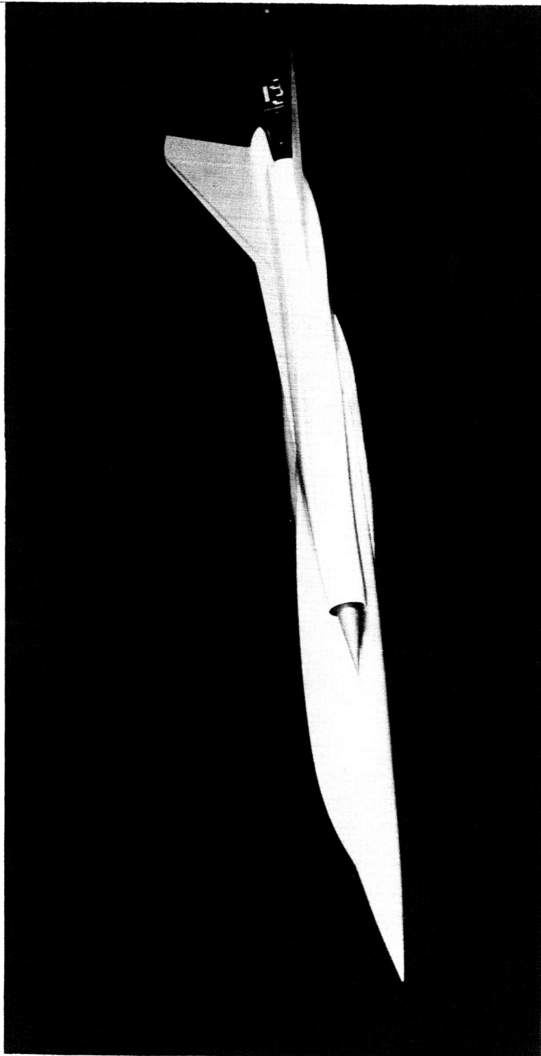
L-60-2015 Figure 9.- Configuration VIIA with reconnaissance pod tested in Langley 8-foot transonic pressure tunnel.
