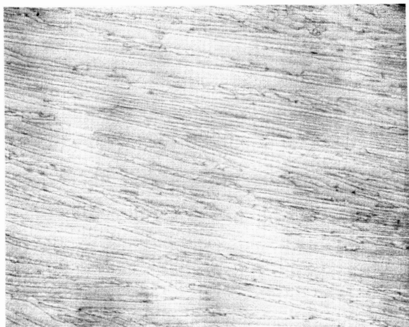
Fig. 1 Longitudinal section of controlled Ni-Ni 3 Nb eutectic 250X.
