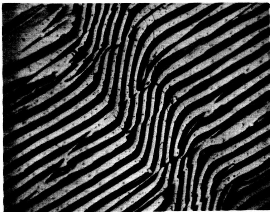
Figure 5. Kink- Band in Al-CuAl 2 with some unbroken CuAl 2 Platelets. 500X
