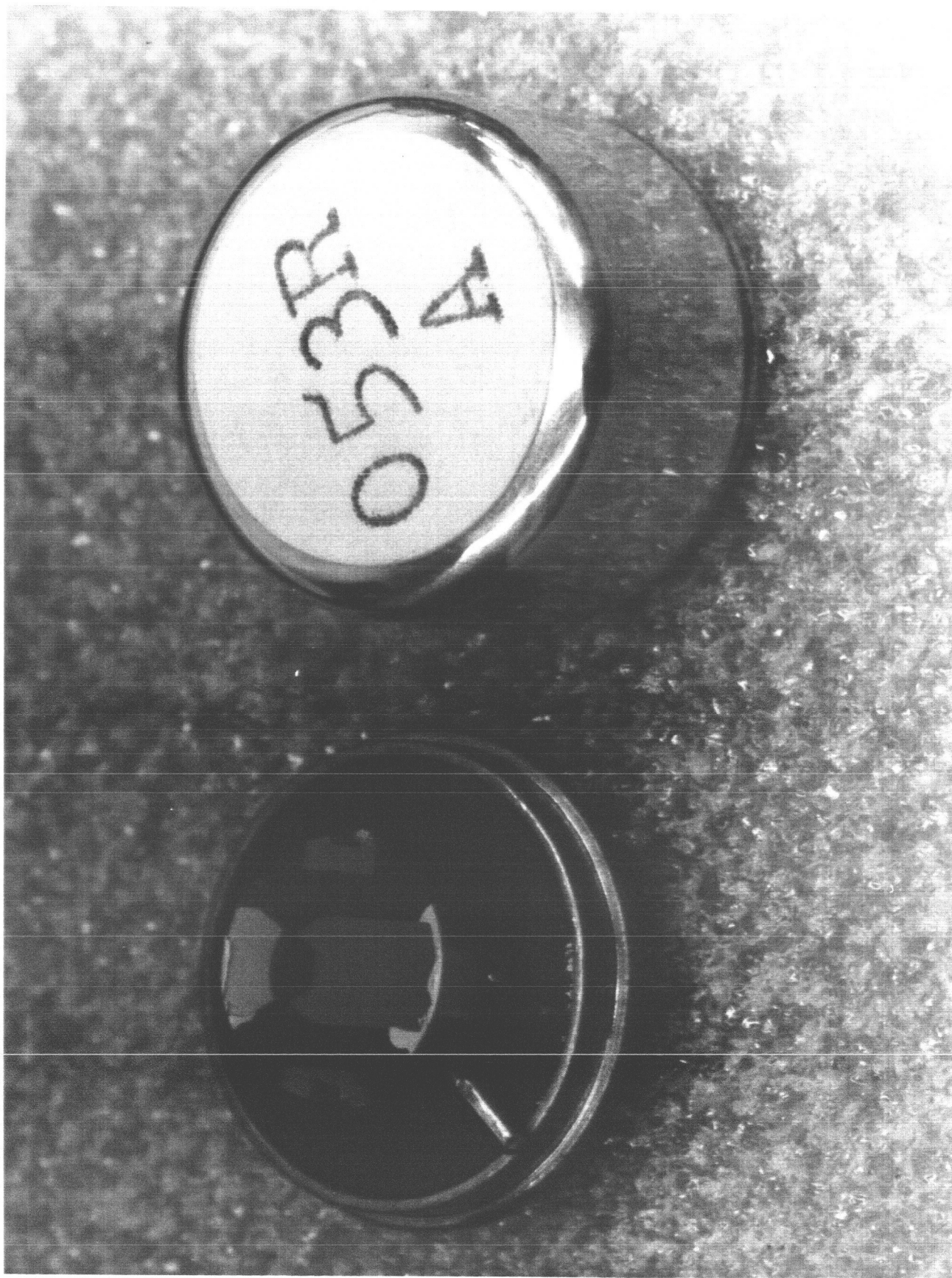
Fig. 21. Mounted composite resonator - unsealed and sealed.
