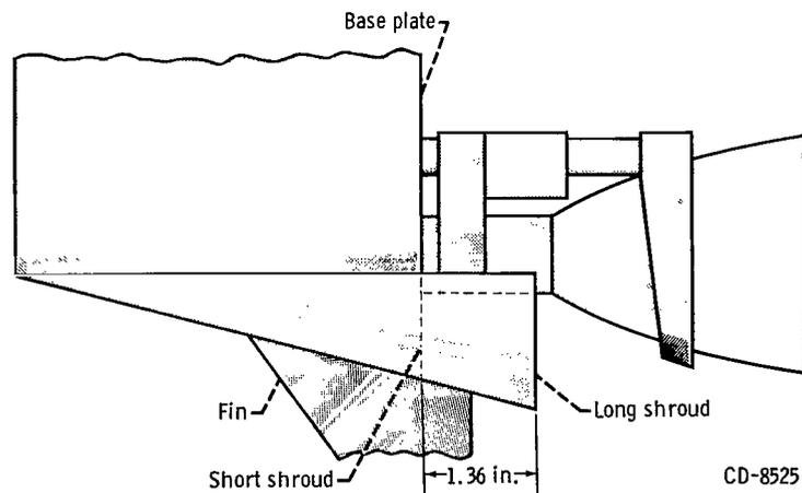
Figure 6. - Comparison of long and short engine shrouds.
