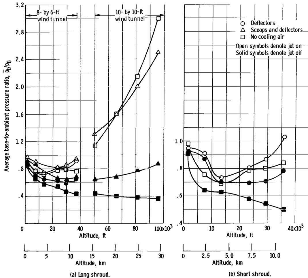
Figure 16. - Effect of cooling air on base pressure.
