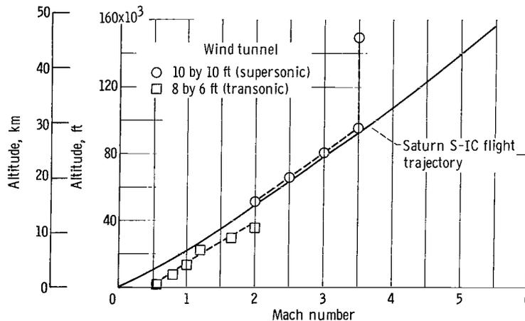
Figure 1. - Comparison of flight and model trajectory.
