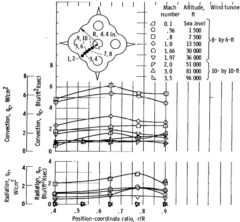
Figure 8. - Typical base-plate heat-transfer distribution. Long shroud; no-cooling-air configuration; hydrogen turbine exhaust.
