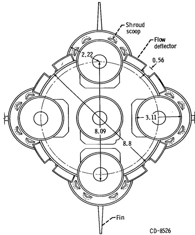
Figure 4. - Comparison of full-scale and model F-1 engine geometry.
