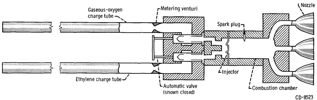
Figure 3. - Schematic drawing of shock-tube combustor.
