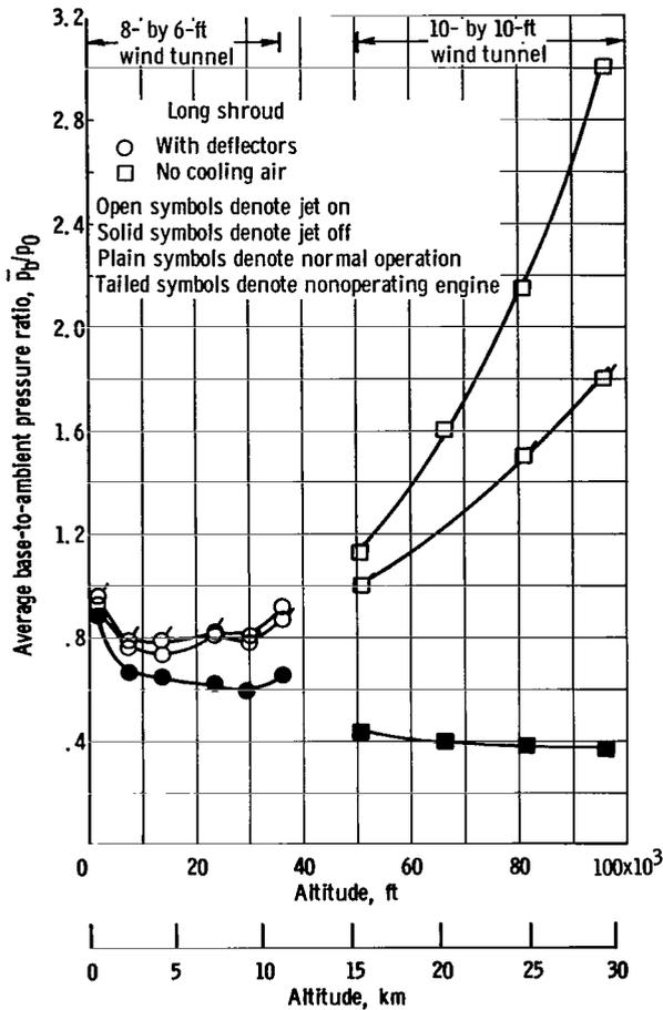
Figure 17. - Effect of engine out on base pressure.
