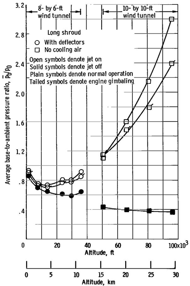
Figure 18. - Effect of nozzle gimbal on base pressure.
