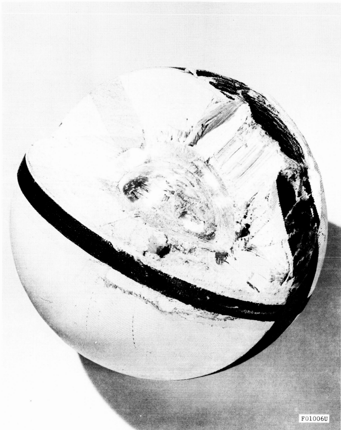
FIGURE A-15. PROTOTYPE PENETROMETER WITH BALSA SLICE REMOVED
