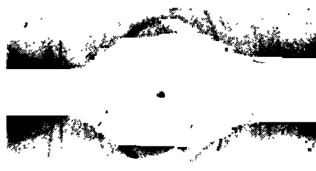
FIGURE 4.—Iron filtered CoK\alpha x-ray pattern of graphite partly converted to diamond by a 300-kbar shock. While the graphite is polycrystalline and randomly oriented, the diamond shows preferred orientation.
