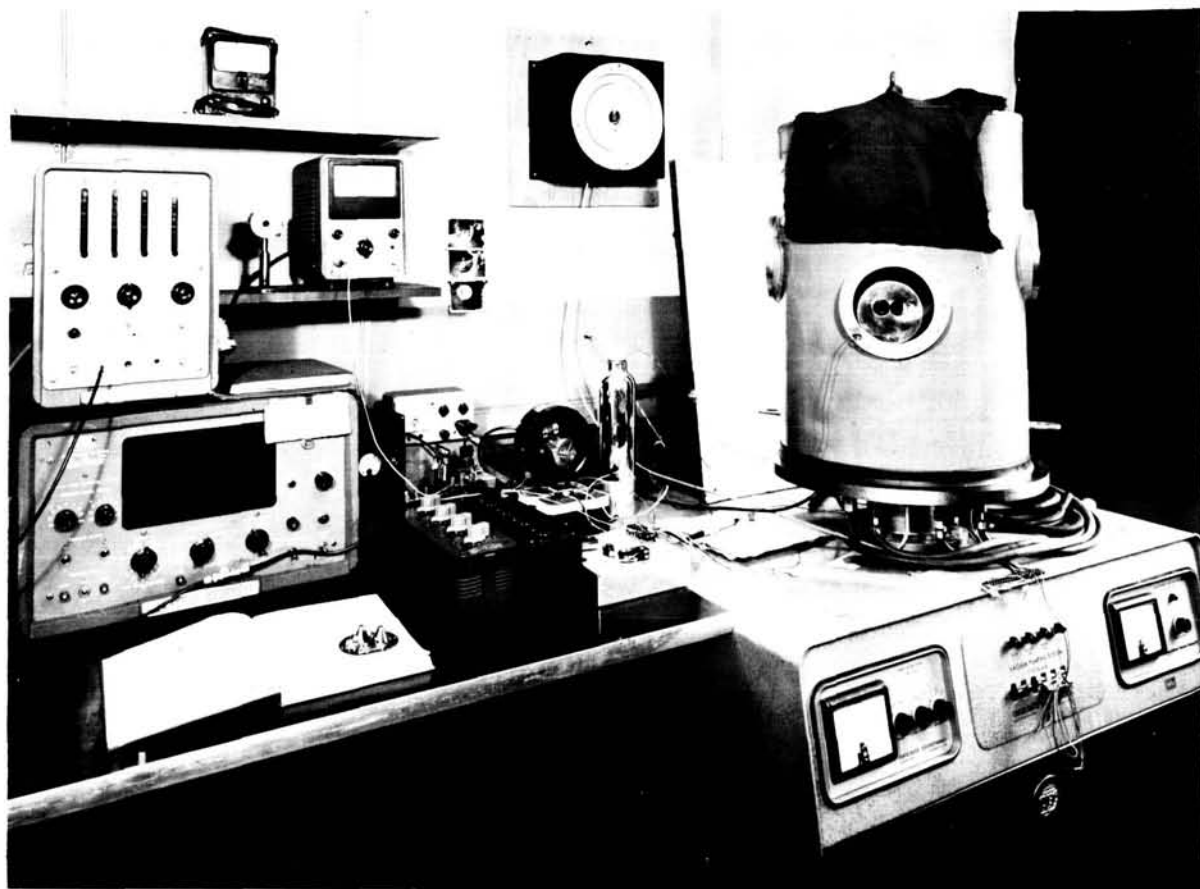
FIGURE 7.—The calibration stand and vacuum chamber. The radiometer mounted for the reflected solar radiation calibration can be seen through the quartz window of the vacuum chamber.
