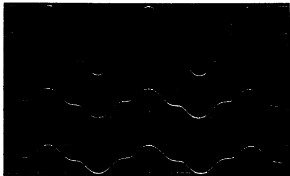
FIGURE 5.—Phase detector bi-directional conduction in the absence of reference input. F=50 kc. Upper trace—1 v RMS signal at Q-6; 1 v p-p=.9 cm. Center trace—output at B 1 , 1 v p-p=1.8 cm. Lower trace—output at B 2 , 1 v p-p=1.8 cm.
