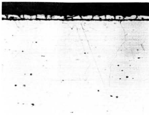
FIGURE 11.—Photomicrograph showing the absence of any reaction of the in situ process to 316SS. Mag. 360X, Marbles etch.
