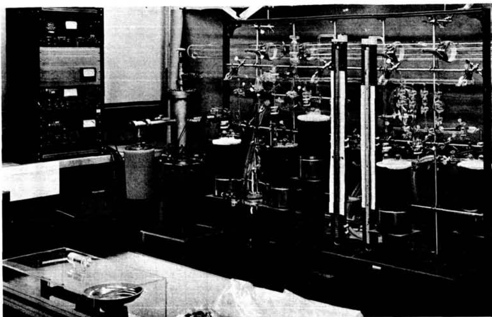
FIGURE 2.—Pressure division calibration system.
