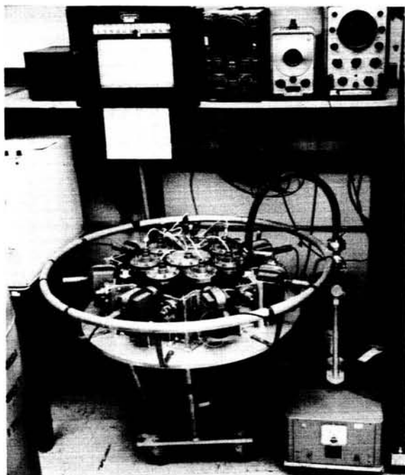
FIGURE 3.—Vacuum system, bearing test program.
