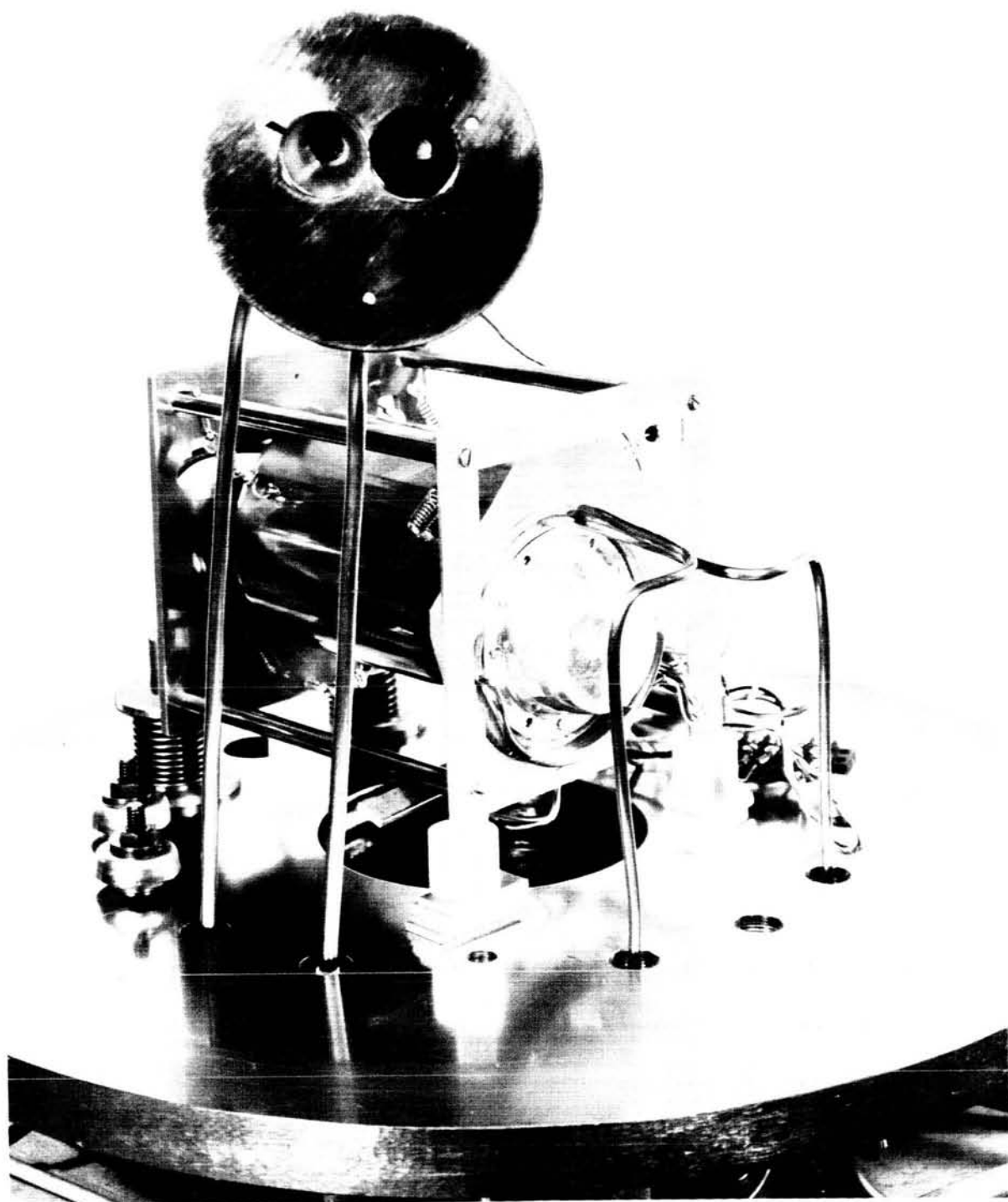
FIGURE 6.—The laboratory calibration apparatus. A low resolution radiometer is positioned in front of the black-body cavity. The upper part of the photograph shows a second radiometer in position for the reflected solar radiation calibration.
