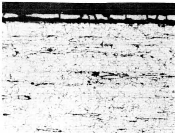
FIGURE 10.—Photomicrograph showing the absence of any reaction of the in situ processing to 416SS. Mag. 360X, hydrofluoric picral etch.
