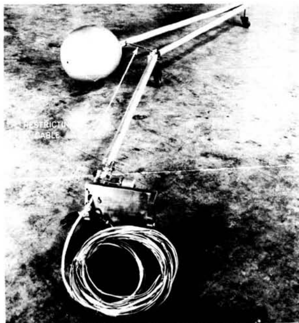
FIGURE 2.—Boom deploying. This illustrates the feature which prevents an experiment from hitting the boom during opening.
