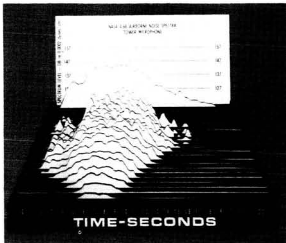
FIGURE 32.—Front view of the three-dimensional plot of NASA 4.68 overall noise level and one-third octave analysis—tower microphone 10.0 kc LPOF.
