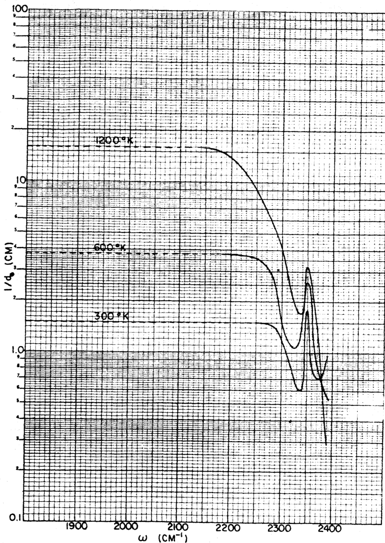
Fig. 8. Values of the line density parameter 1/d_0 for the 4.3- \mu band of \text{CO}_2 . The dashed portions of the curves are extrapolated values. These data are tabulated in Table I.
