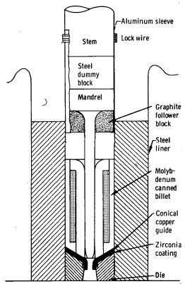
Small-diameter, thin-wall seamless tubing of the refractory metal tungsten has been fabricated in lengths of up to 10 feet by hot extrusion over a floating mandrel. Successful extrusion of 0.50-inch-diameter tubing over 0.4-inch-diameter mandrels was accomplished at temperatures ranging from 3000° to 4000° F. Tubing of 0.375-inch diameter was extruded successfully over 0.3-inch-diameter mandrels at 3500° and at 4000° F.
