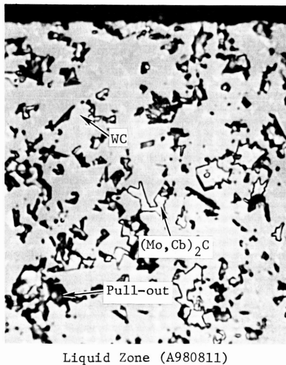
Figure 20. Microstructure of Transverse Sections of Grade 7178 After Exposure With Mo-TZM Alloy to Potassium for 1000 Hours at 1200°F.
