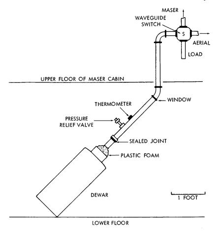
Fig. 3 — Layout of cold load at Goonhilly.
