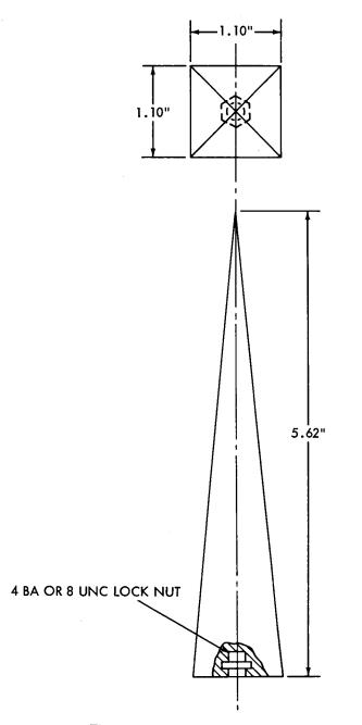
Fig. 2-Poly-iron pyramid load,
