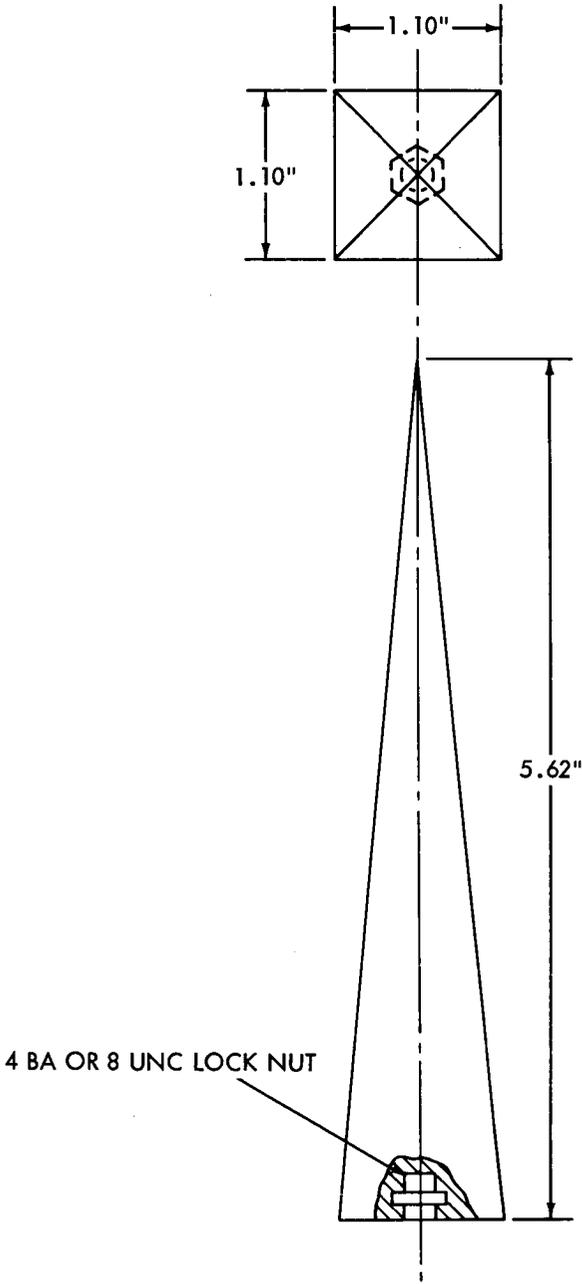
Fig. 2 — Poly-iron pyramid load.
