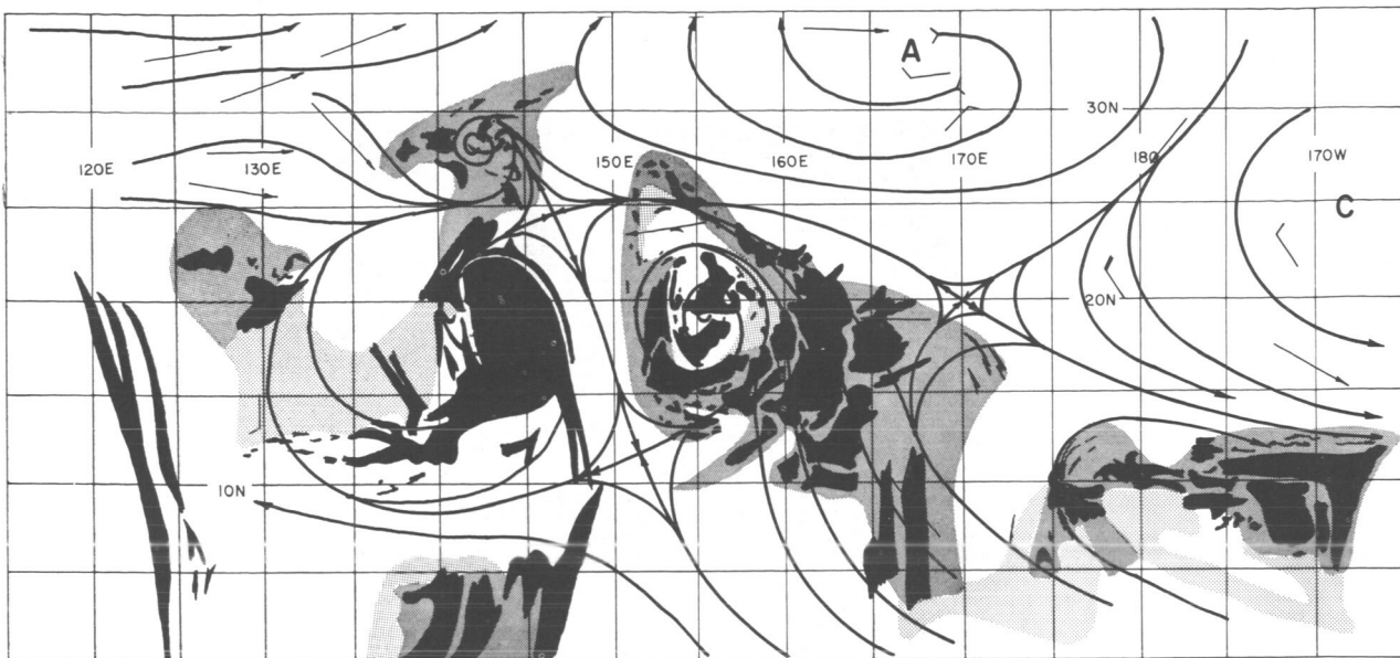
Figure 9-72—HRIR Revised 300 mb Streamline Analysis, 1200 UT, 19 September 1964
