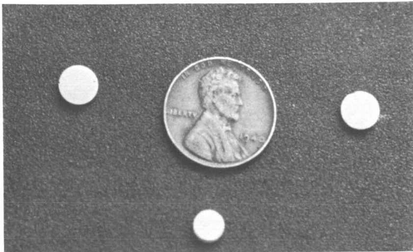
FIGURE 1.—Spore tablets compressed at 30 tons per square inch.
