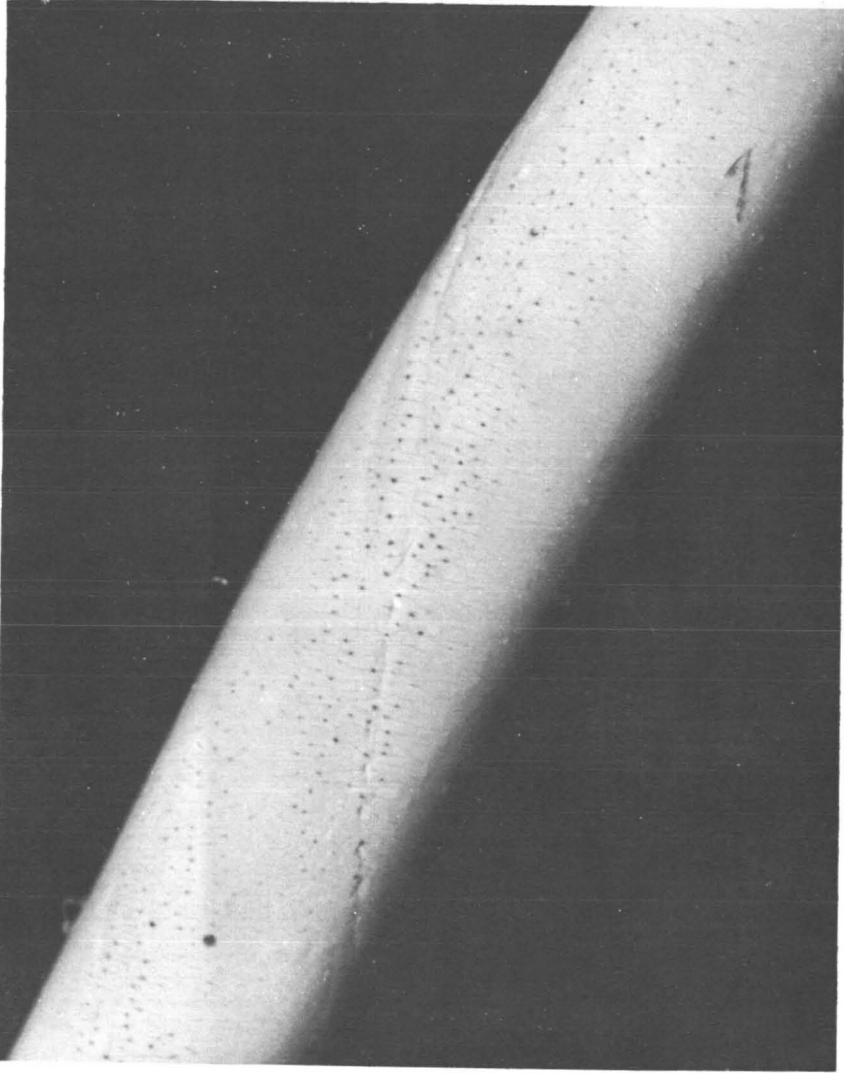
FIGURE 9.—Pinholes and stress lines radiating at right angles to length of wire in hookup wire with FEP over H-film. Color, white; conductor No. 16.
