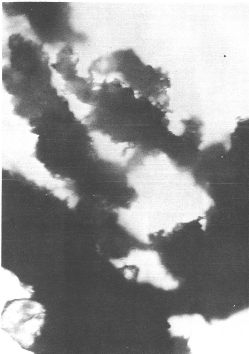
FIGURE 5.—Microphotograph of solid rocket propellant particles in water demonstrating structure of binder. Most crystals of ammonium perchlorate have been dissolved, exposing structure of binder.
