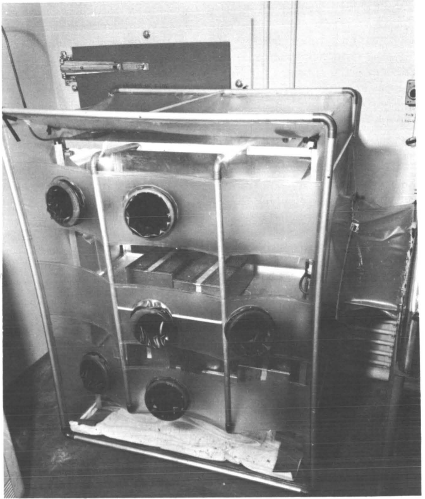
FIGURE 6.—Plastic enclosure for an animal cage rack.
