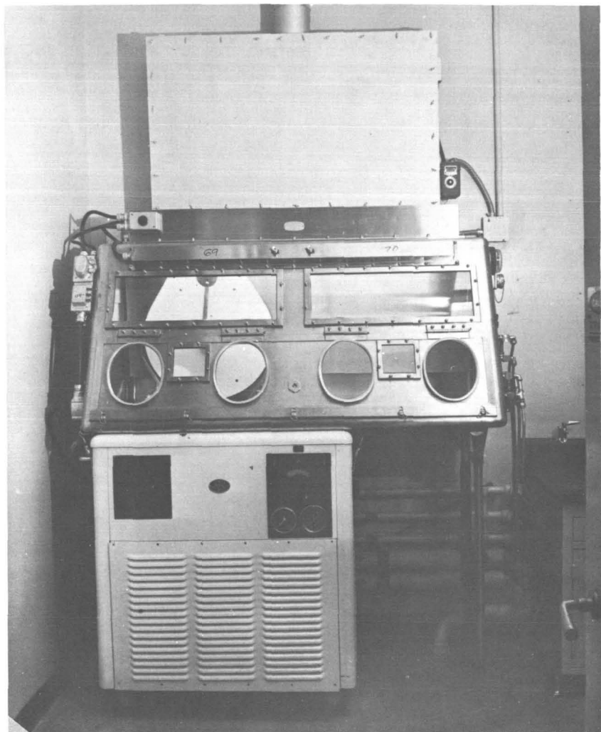
FIGURE 11.—Microbiological cabinet for centrifuge operations.
