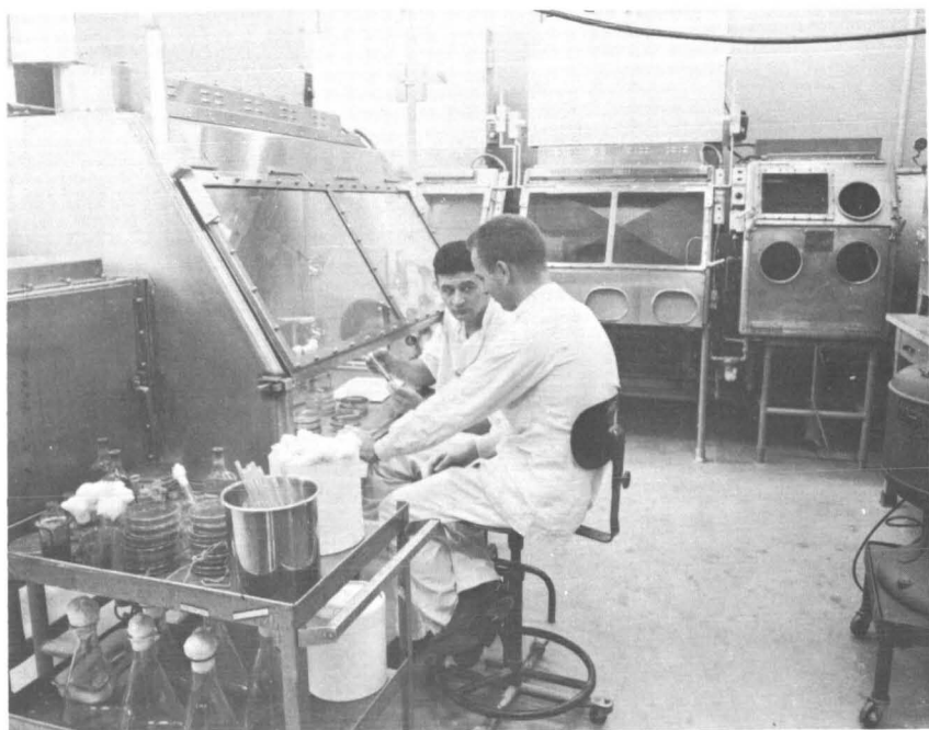
FIGURE 9.—Open-panel microbiological safety cabinets.
