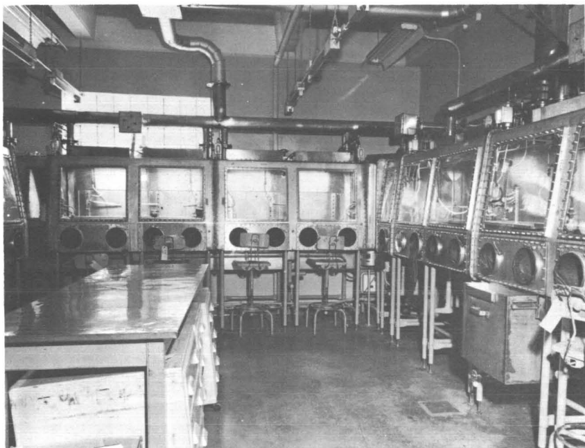
FIGURE 17.—Large gastight cabinet system for laboratory operations.
