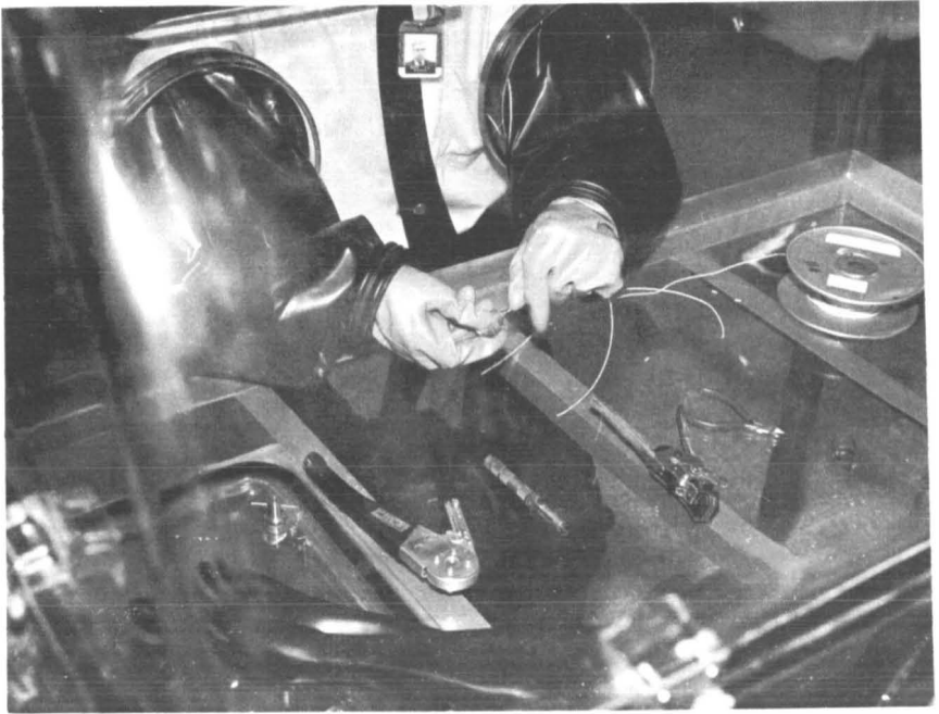
FIGURE 7.—Removal of pin from connector.
