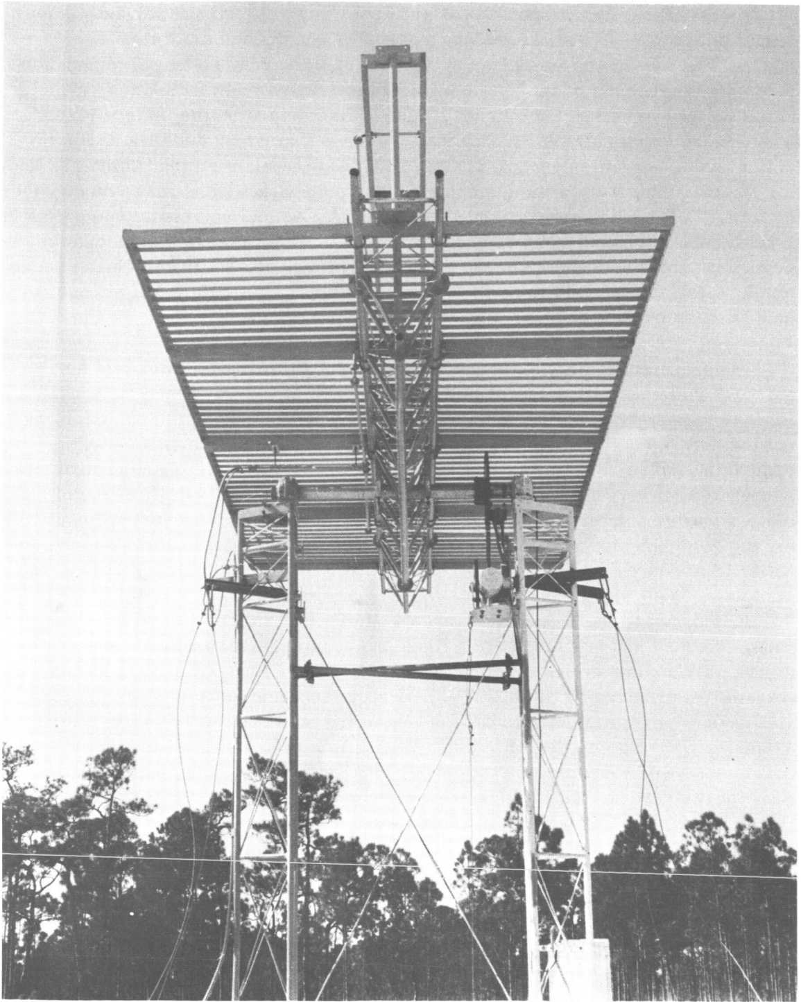
Figure 7. Photograph of the "rockinghorse" data-acquisition antenna deployed around the Mini-track network during the IGY. The antenna portion—the part that "teeters"—is just a section of the regular interferometer antenna. (Courtesy of W. Mitchell, GSFC)
