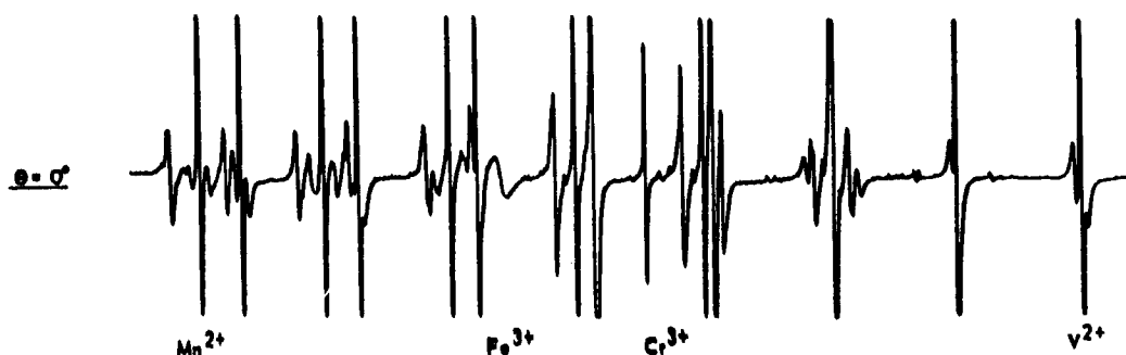
Fig. 2.3. ESR spectra of \text{V}^{4+} , \text{Cr}^{3+} , \text{Mn}^{2+} and \text{Fe}^{3+} in a single crystal of \text{CaO} at \theta = H \wedge [100] = 0 and T = 300^\circ\text{K}
