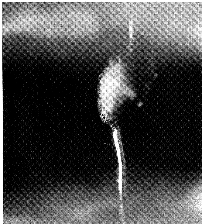
Fig. 2. Photograph showing enlarged thermistor and wires before painting (magnification = 150)
