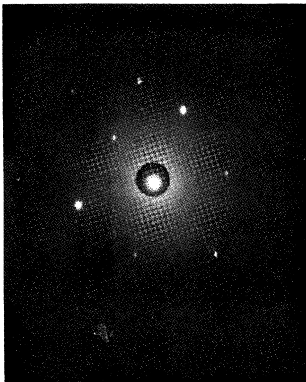
(a) Single-crystal copper before experiment.
