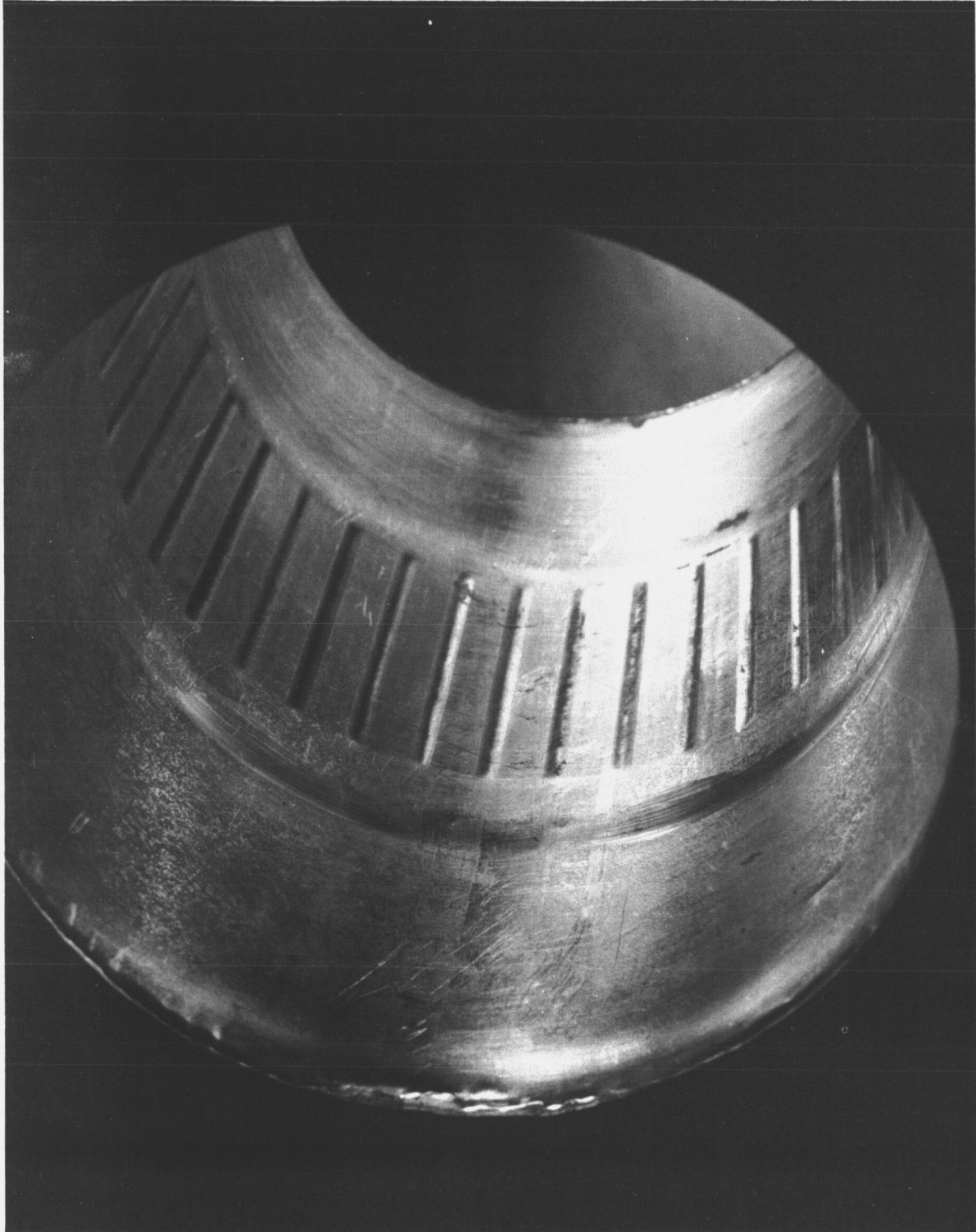
NaK Pump-Motor Stator Housing (P/N 092992-1) from INL-3 Unit 2/3 - Recirculation Pump End
