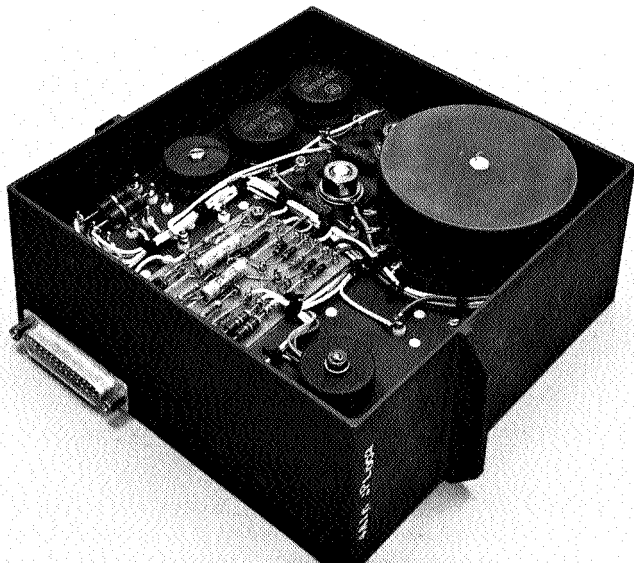
Fig. 2. Typical 6- × 6-in. electronic subchassis
