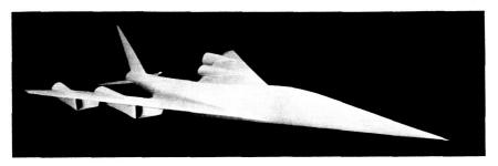
Outlines a construction method by which wind-tunnel models of both simple and complex configuration can be produced rapidly at reduced cost. An interesting casting and plasticizing technique developed by Langley Research Center that may be applied to items not necessarily related to the aircraft industry.
