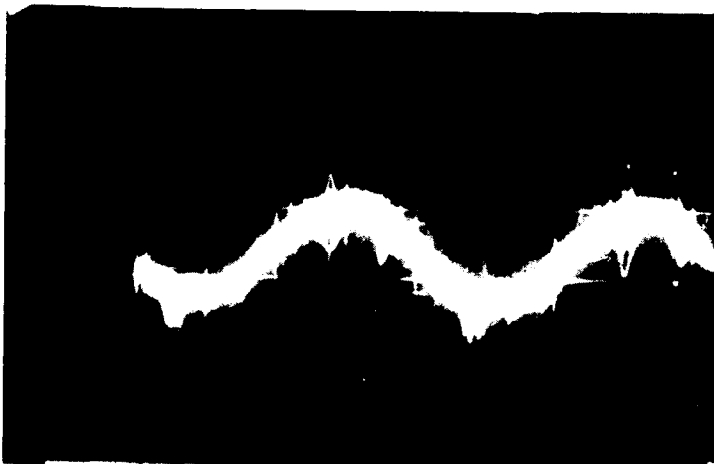
II.8 Demodulated sine wave [multiple exposure] for an FM signal via a fading channel. \beta=12.5 , 2kHz modulating signal. 0.5 rpm rotation of the multipin scatterer.
