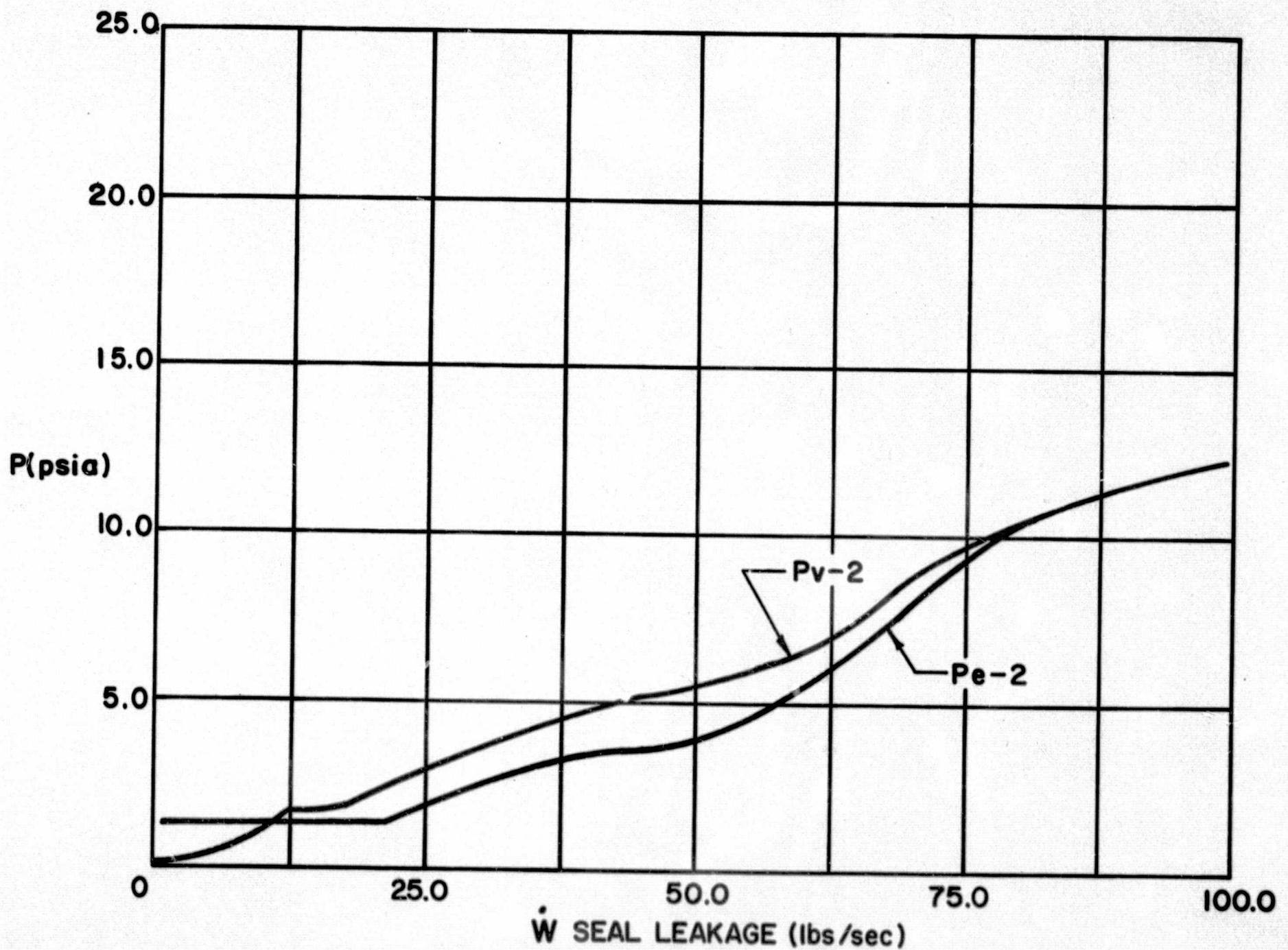
NOZZLE EXIT AND ENGINE COMPARTMENT PRESSURES
