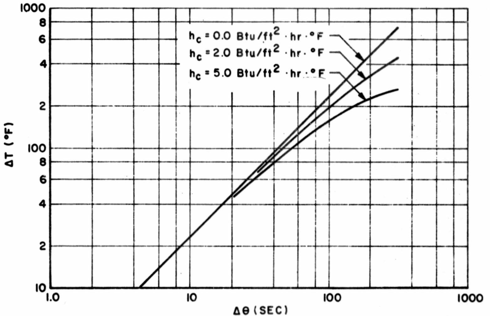
TEMPERATURE RISE ( $\Delta T$ ) FOR 14 GAGE (0.064 in. THICK) SHEET ALUMINUM RECEIVING A CONSTANT RADIATIVE HEAT FLUX OF  $2.0 \text{ Btu/ft}^2 \cdot \text{SEC}$  AS A FUNCTION OF TIME ( $\Delta\theta$ ) AND ADJACENT AIR CONVECTION COEFFICIENT ( $h_c$ )
