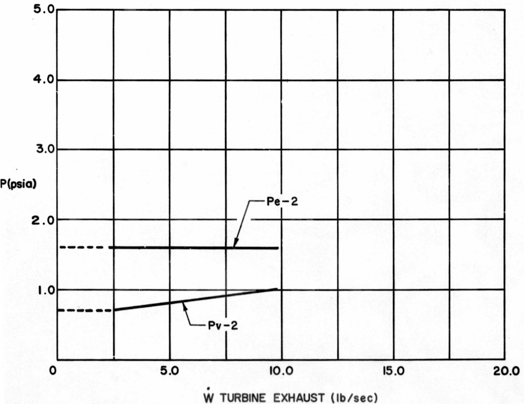
**NOZZLE EXIT AND ENGINE COMPARTMENT PRESSURES
