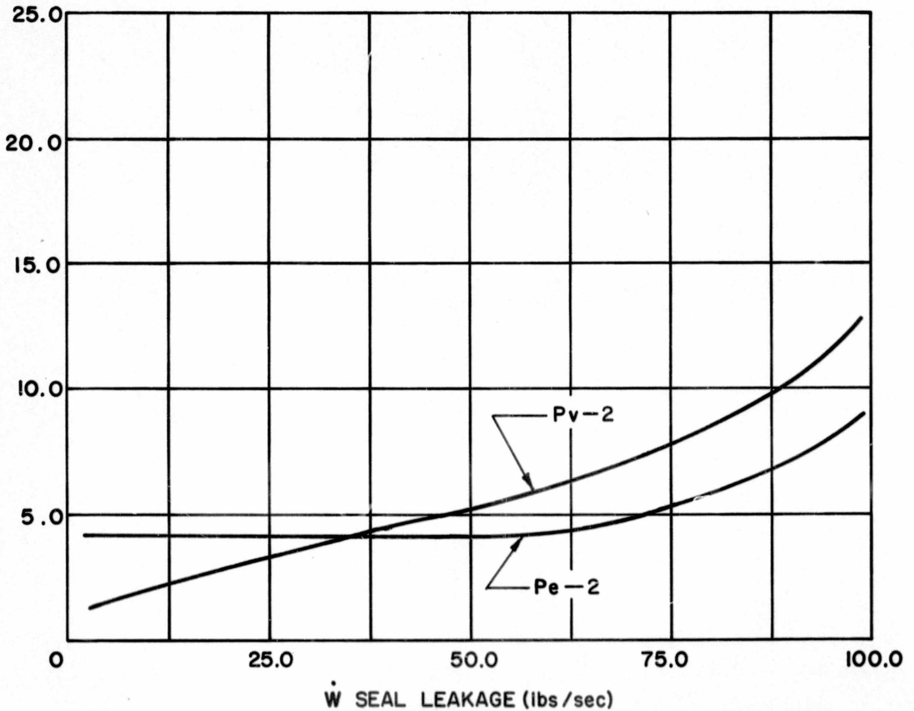
**NOZZLE EXIT AND ENGINE COMPARTMENT PRESSURES
