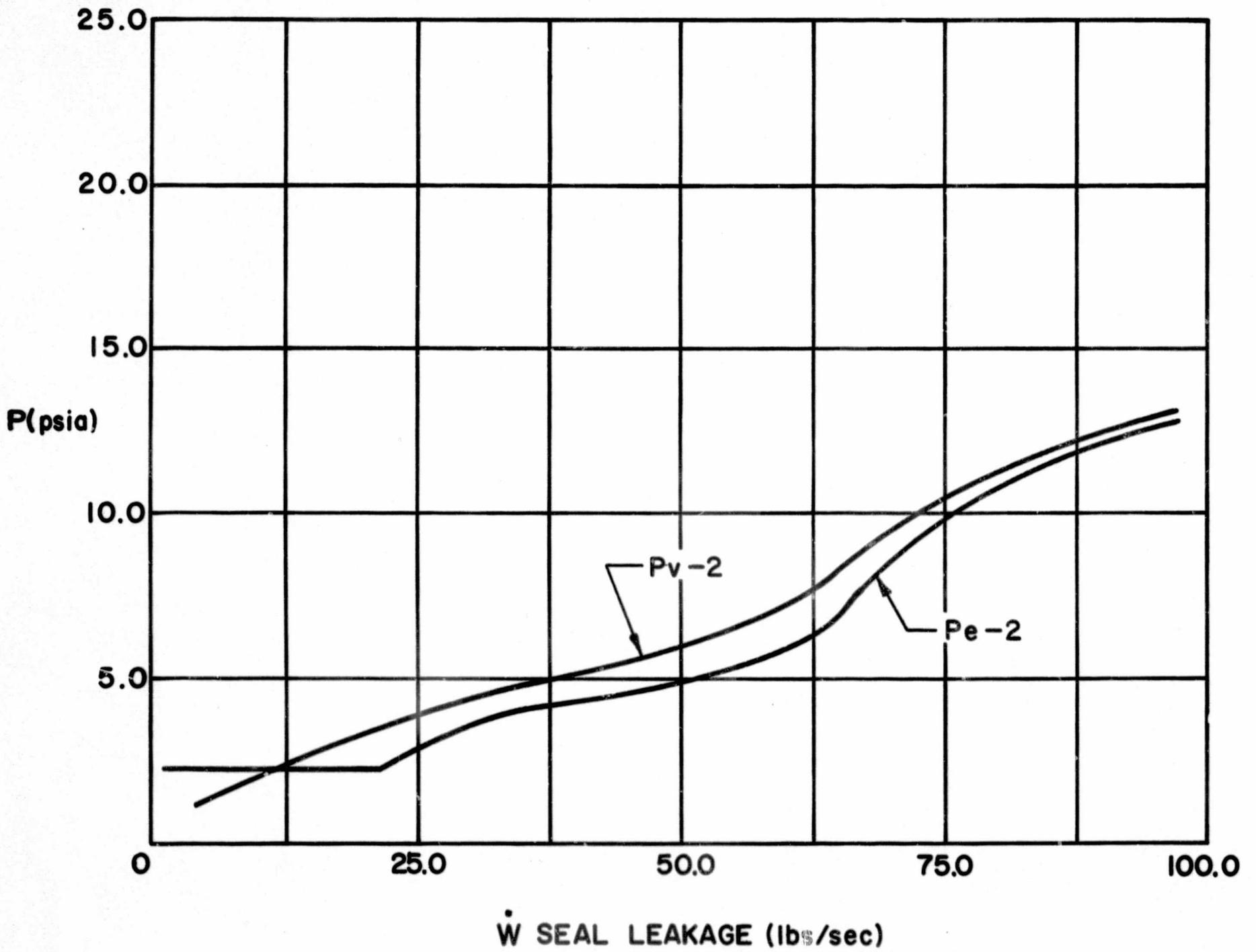
**NOZZLE EXIT AND ENGINE COMPARTMENT PRESSURES
