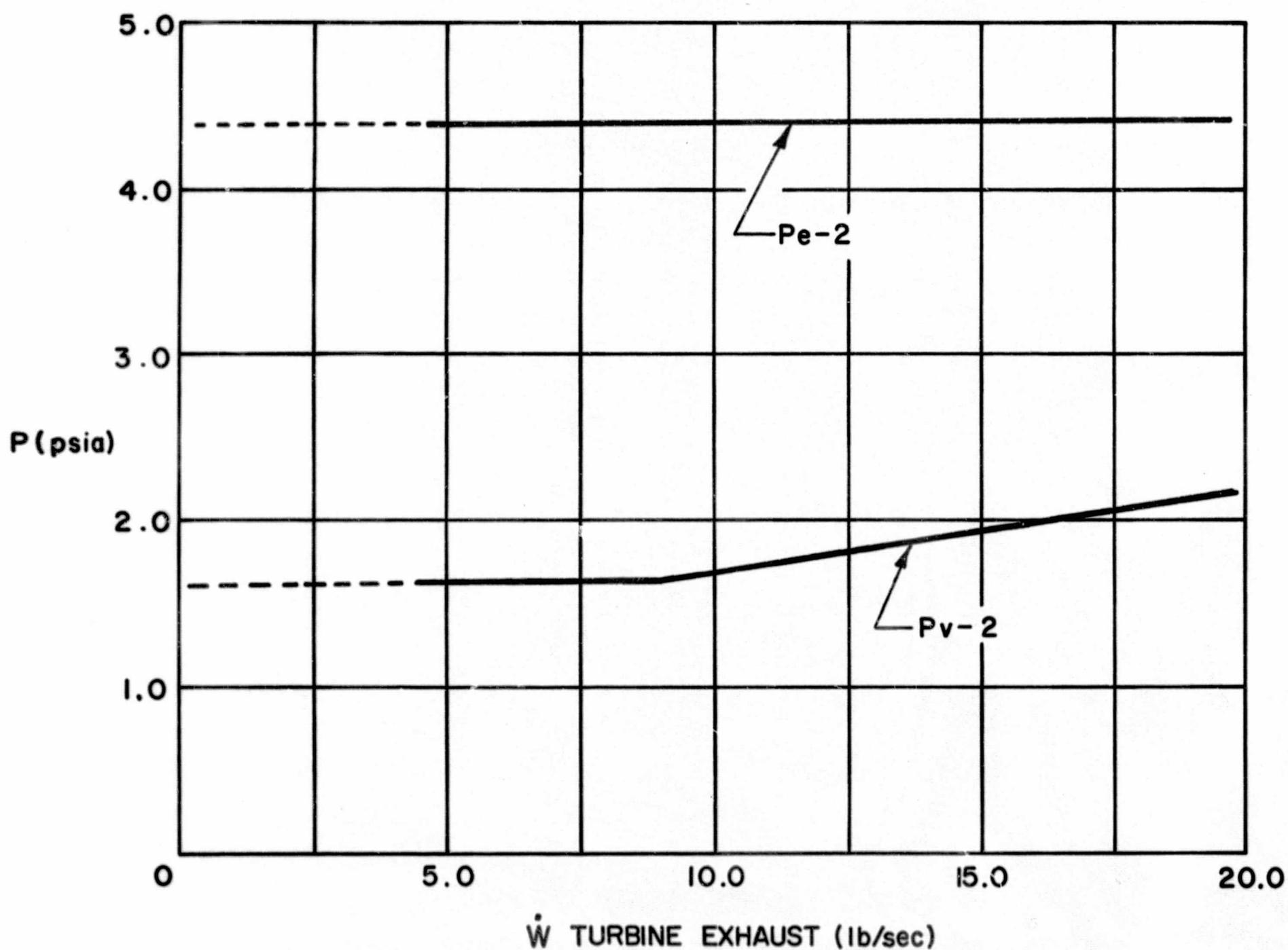
**NOZZLE EXIT AND ENGINE COMPARTMENT PRESSURES
