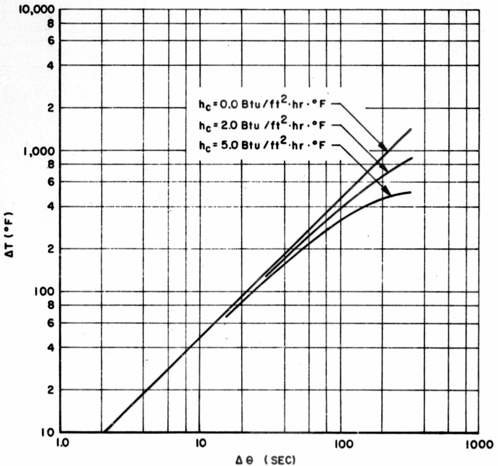
**TEMPERATURE RISE ( $\Delta T$ ) FOR SHEET ALUMINUM (14 GAGE) RECEIVING A CONSTANT RADIATIVE HEAT FLUX OF 4.0 Btu/ft<sup>2</sup> SEC AS A FUNCTION OF TIME ( $\Delta \theta$ ) AND ADJACENT AIR CONVECTION COEFFICIENT ( $h_c$ )**
