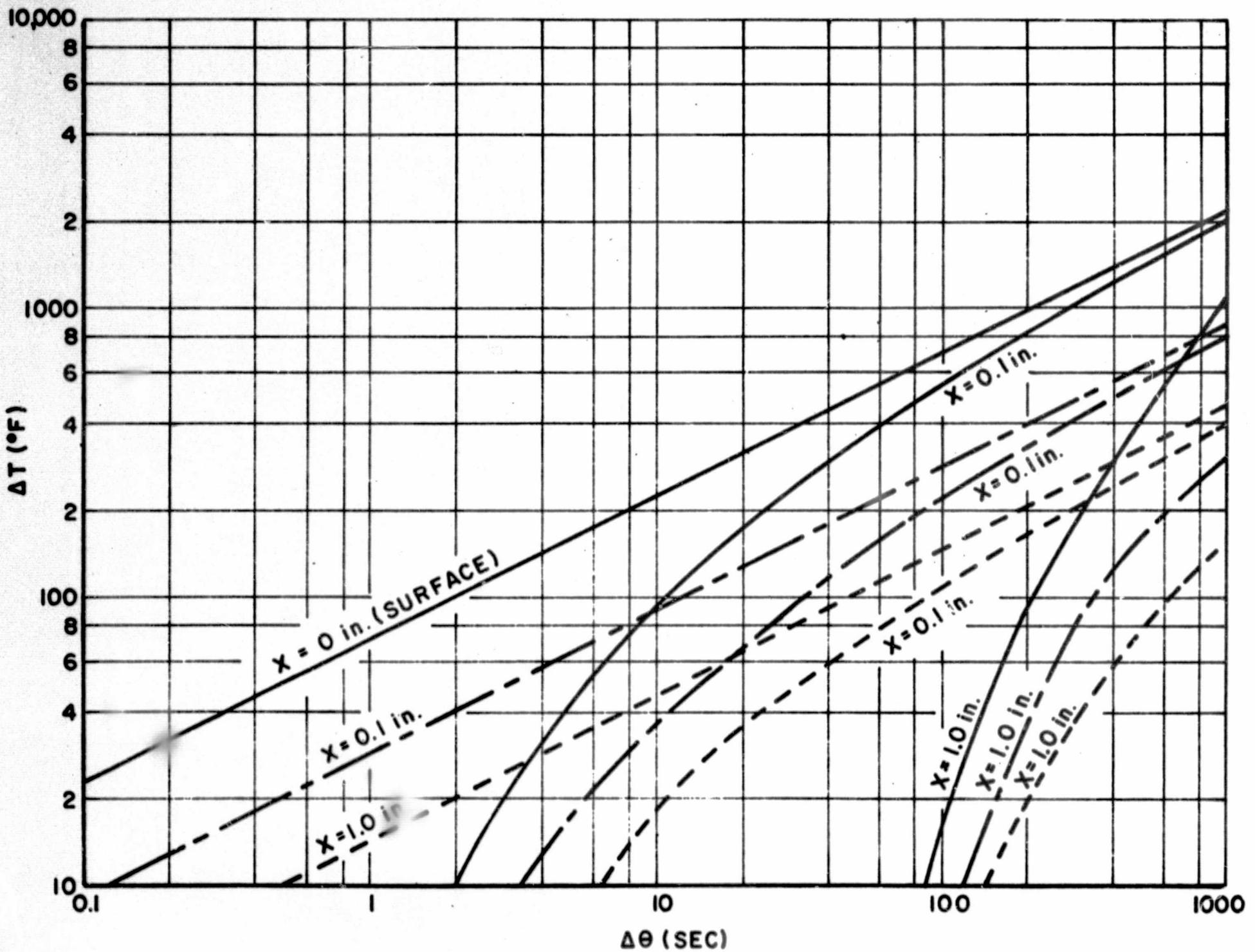
**TEMPERATURE RISE FOR SEMI-INFINITE CONCRETE SLAB AS A FUNCTION OF DISTANCE (X) FROM SLAB SURFACE AND TIME INCREMENT ( $\Delta\theta$ ) FOR RADIATIVE HEAT FLUXES  $q/A = 1.0, 2.0, \& 5.0 \text{ Btu/ft}^2 \cdot \text{sec}$**
