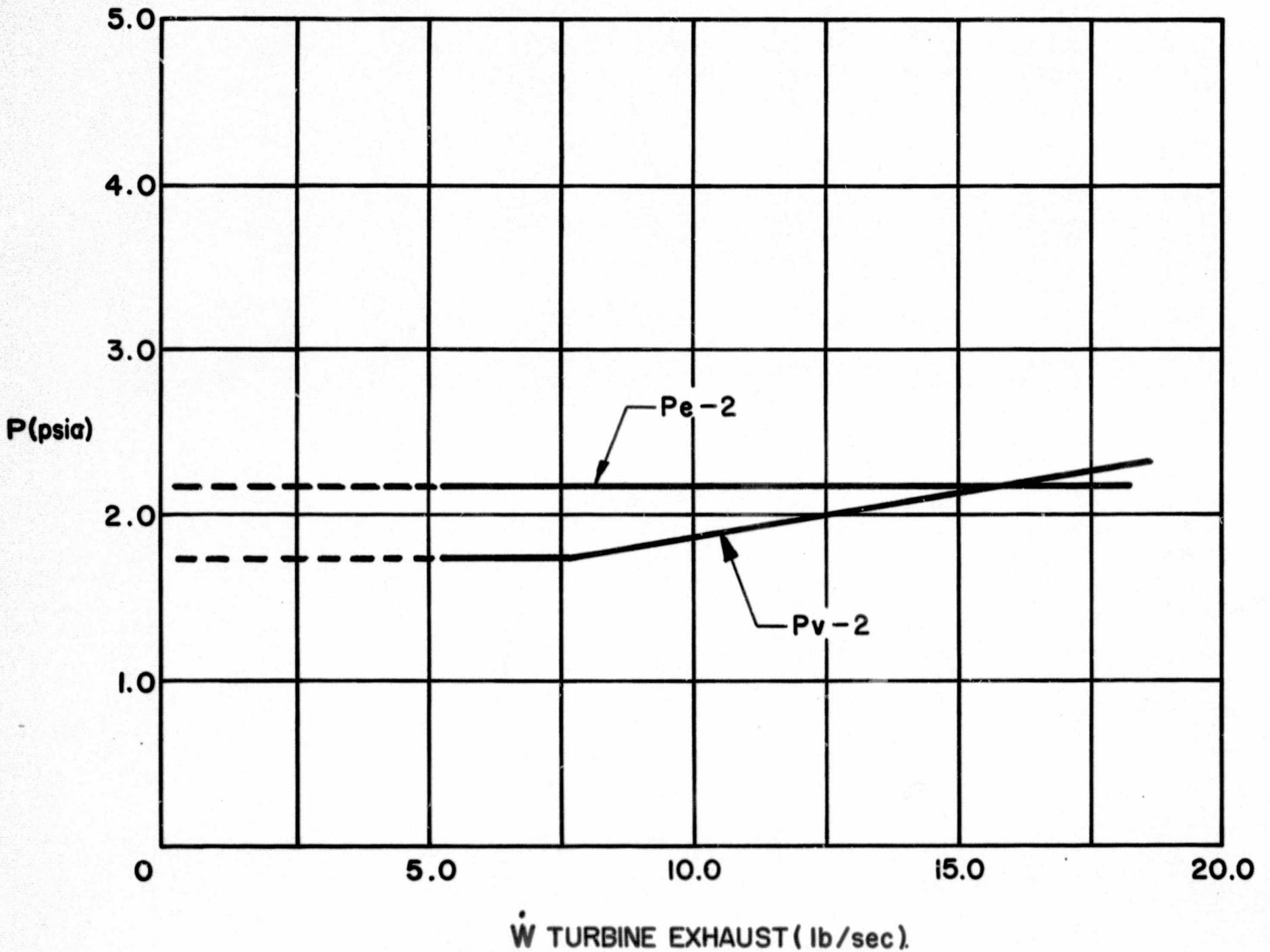
NOZZLE EXIT AND ENGINE COMPARTMENT PRESSURES
