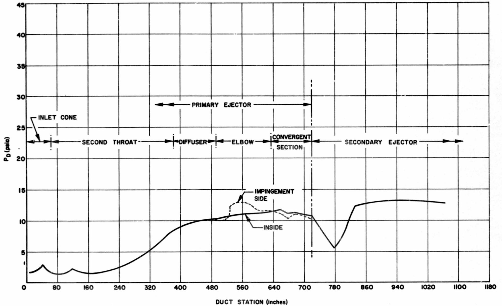
**EJECTOR WALL PRESSURES WHEN TESTING THE 12/1 NOZZLE
