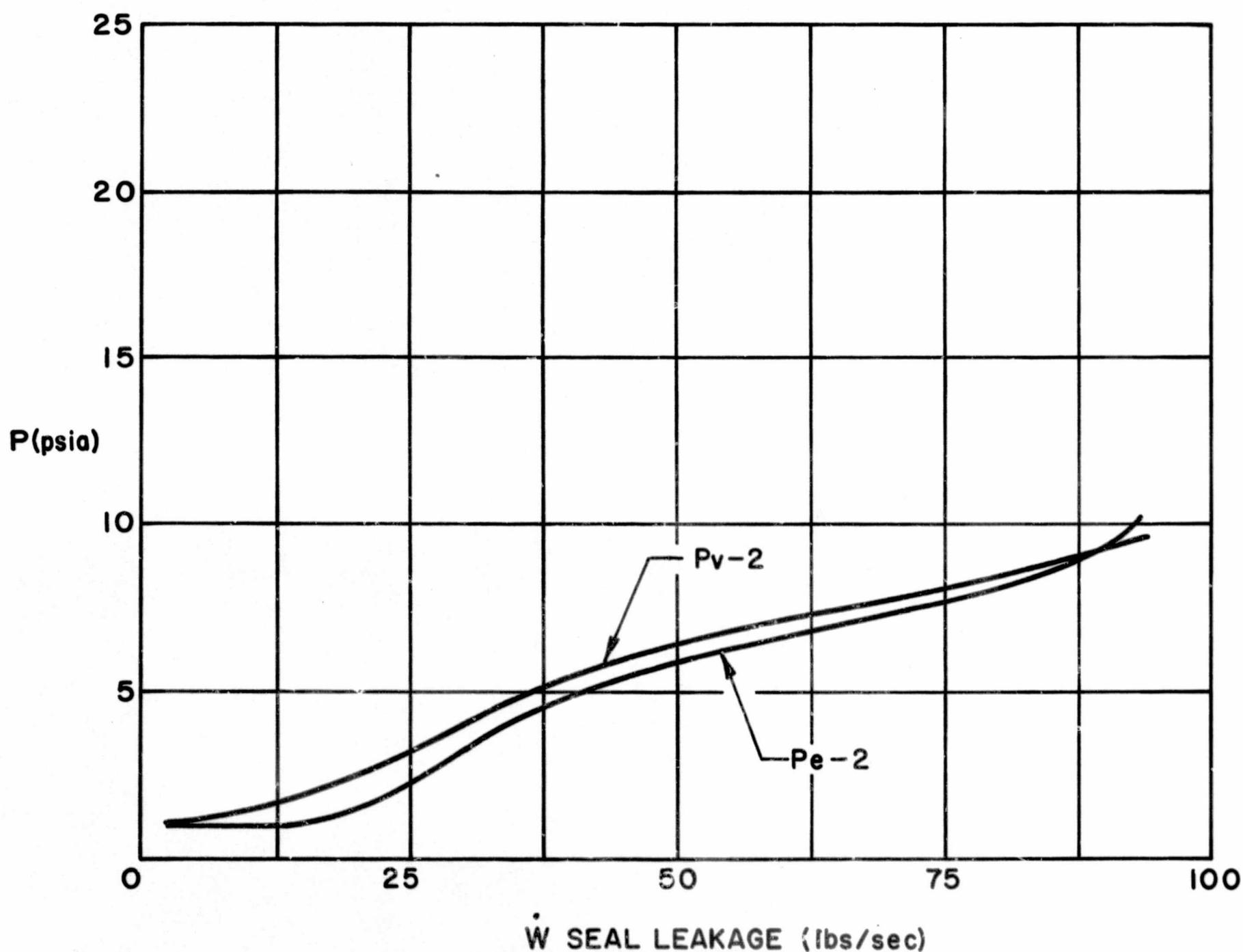
**NOZZLE EXIT AND ENGINE COMPARTMENT PRESSURES
