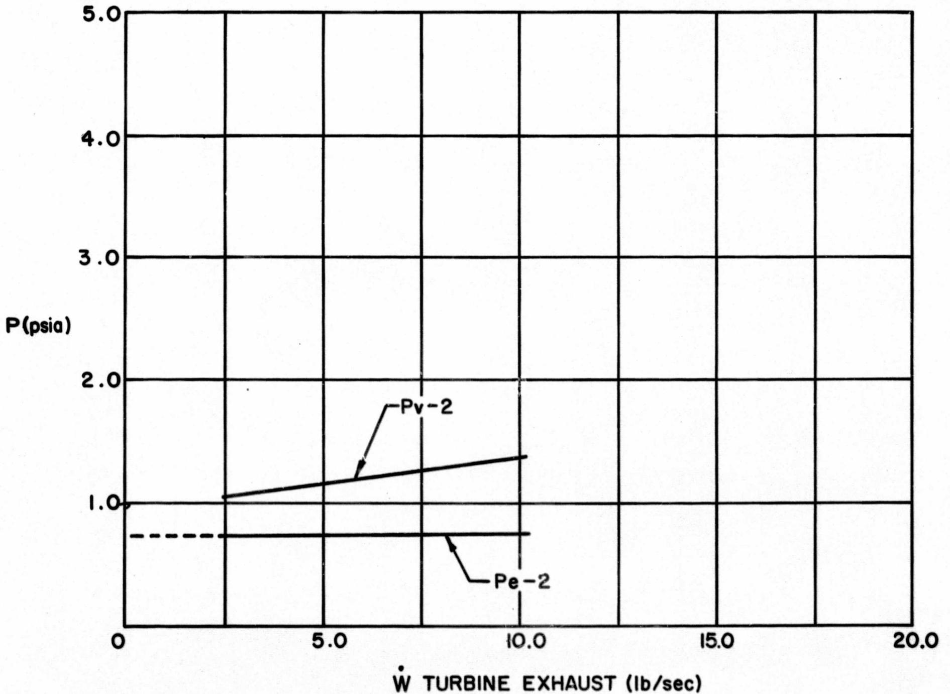
**NOZZLE EXIT AND ENGINE COMPARTMENT PRESSURES
