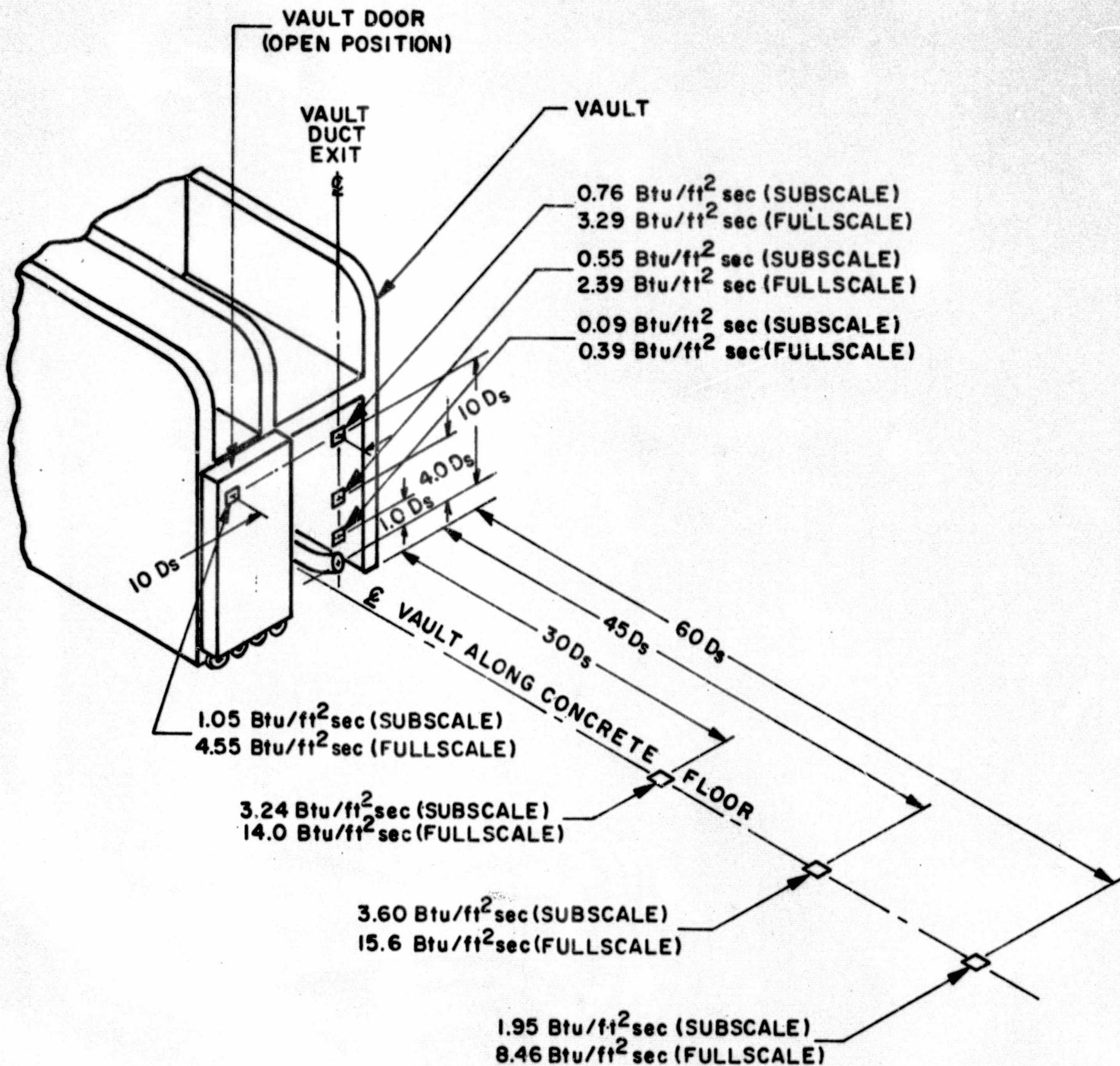
**THERMAL RADIATION FLUX FROM NERVA
