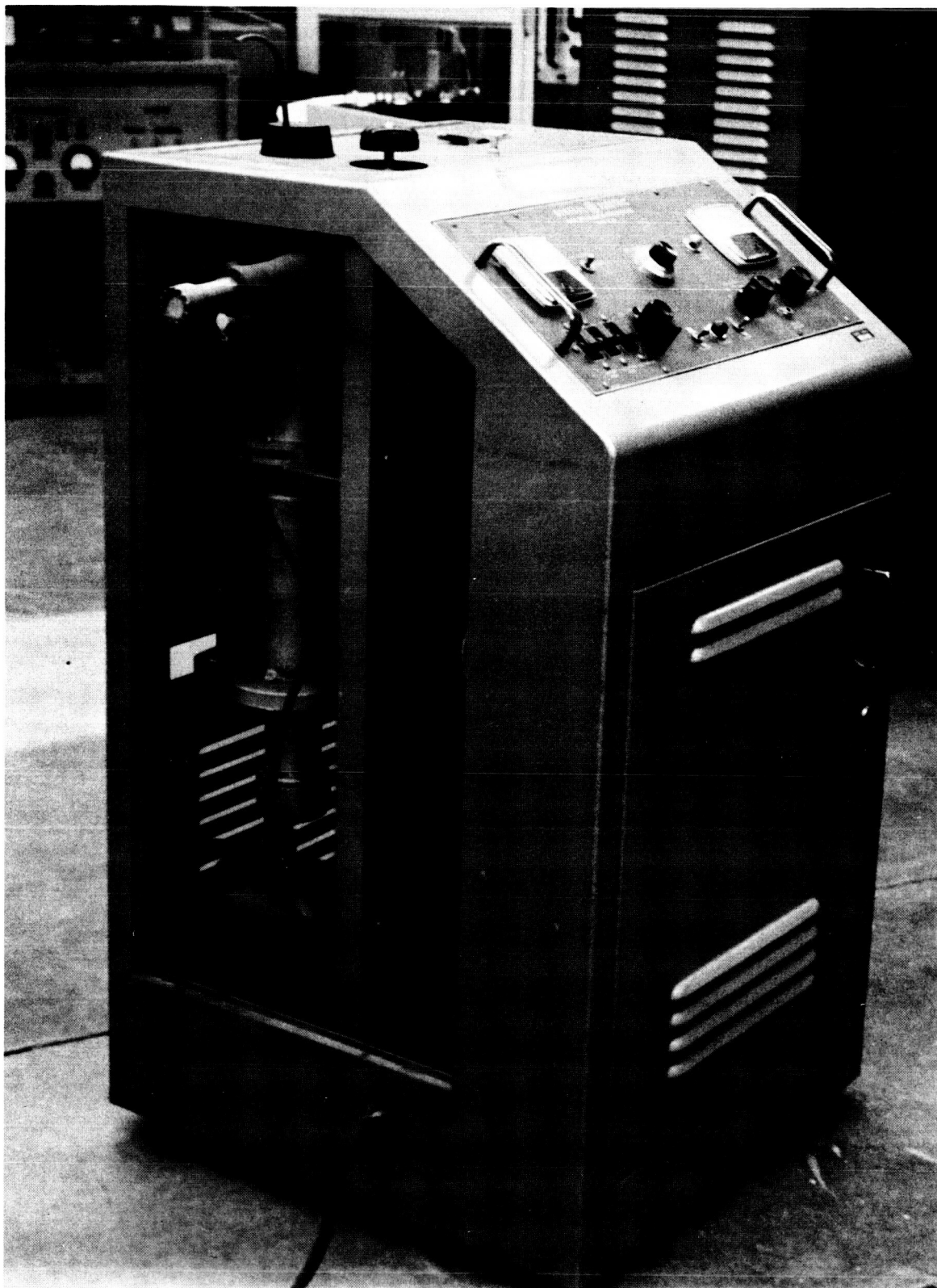
Brass Test Cell With Teflon Membrane Mounted On General Electric Mass Spectrometer, Model M-60
