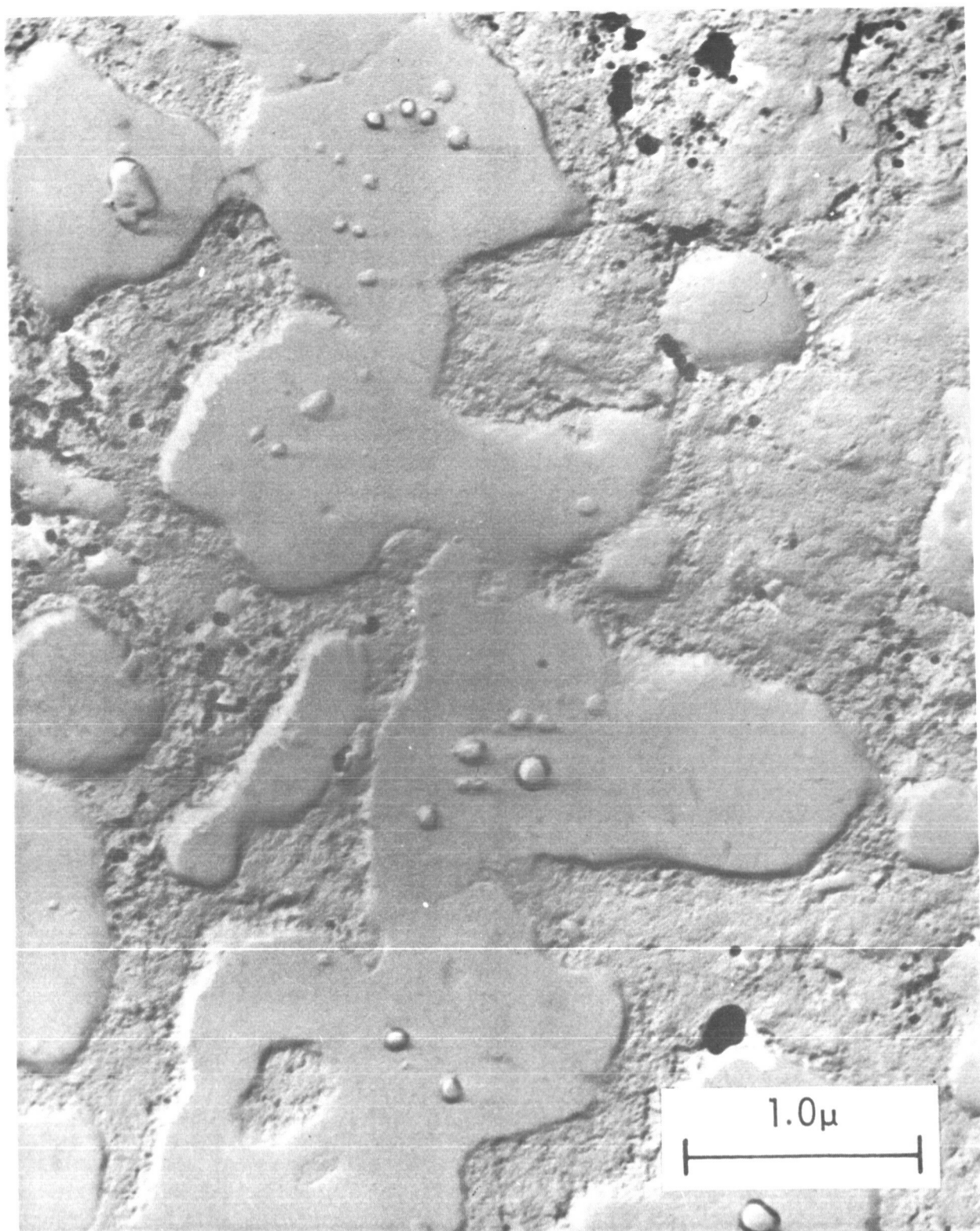
Figure 6. - Electron Micrograph of CR-3.8-Volume-percent-MgO after hydrogen reduction (20,000X).
