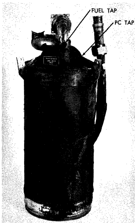
Figure 35—Flight 4.113 GA-GI thrust chamber jacket showing broken pressure chamber and fuel taps.
